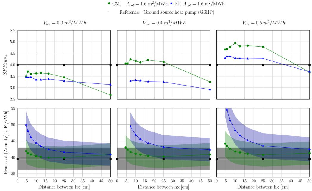
**Fig. 6: System performance (up) and heat generation cost (bottom) as function of the distance between heat exchangers. Three ice storage volumes are used: (left)  $3 \text{ m}^3$ , (mid)  $4 \text{ m}^3$  and (right)  $5 \text{ m}^3$ .**
