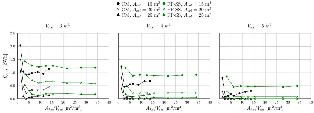
Fig. 4: Direct electric back-up as a function of heat exchanger area divided by ice storage volume for three ice storage volumes of (left)  $2 \text{ m}^3$ , (mid)  $4 \text{ m}^3$  and (right)  $5 \text{ m}^3$ .
