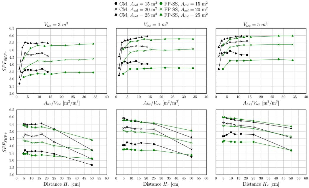
Fig. 3: Yearly system performance as function of (top) heat exchanger area divided by ice storage volume and (bottom) distance between heat exchangers for three ice storage volumes of (left)  $2 m^3$ , (mid)  $4 m^3$  and (right)  $5 m^3$ .
