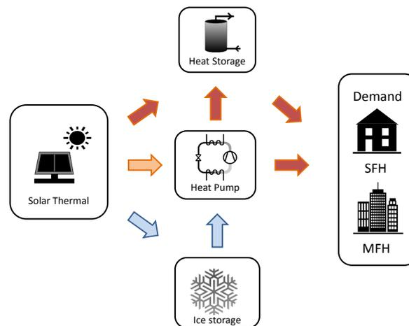
**Fig. 1: Principle concept of solar-ice systems. The arrows show the heat fluxes that are on different temperature levels, i.e. red, orange and blue for high (>30 °C), medium (>10 °C) and cold (<10 °C) respectively.**
