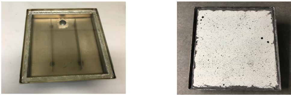
Figure 8. (a) 250mmx250mm fabricated collector with soldered glass, (b) Speckle pattern created on prototype collector
