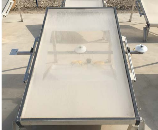
Fig. 4: the two pyranometers are mounted onto an arm that is held by a fixture construction to ensure that the measurements are always at the same position
