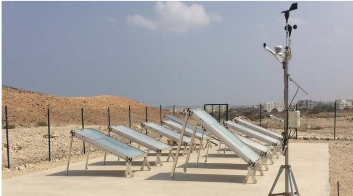
Fig. 1: Overview of the experiment site with eight different transparent covers in their frame, four different PV glass samples and a weather station with temperature and humidity sensor, wind direction and wind velocity sensor
