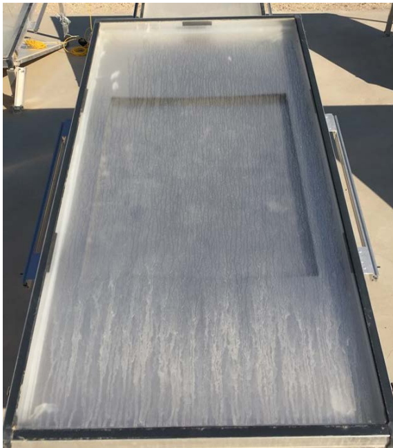
Fig. 5: When dew is forming it can generate droplets that flow down the glass cover. This creates visible flow patterns
