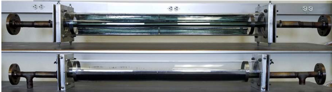
Fig. 11: Thermal receiver after 50 hours of continuous operation.
