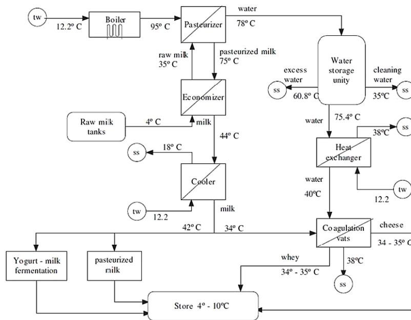
Fig. 1: Adapted scheme of a dairy facility (tw: tap water; ss: sewage system) [9].
