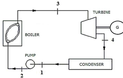
Fig. 4: Simplified scheme of a Rankine cycle.
