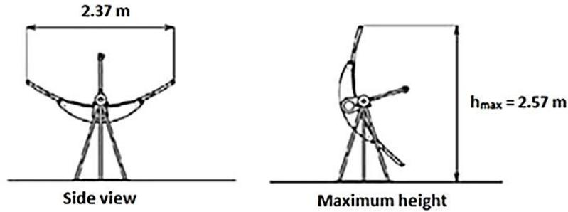
Fig. 2: Section of the collector: maximum width and height [11].
