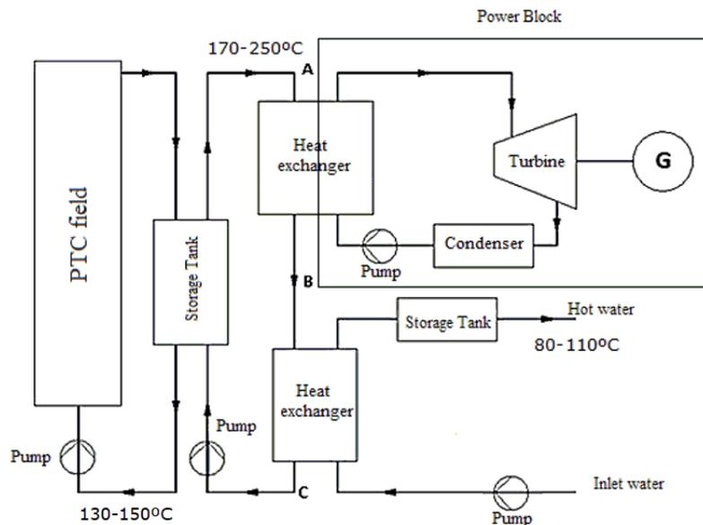
Fig. 3: Simplified scheme of a cogeneration system.
