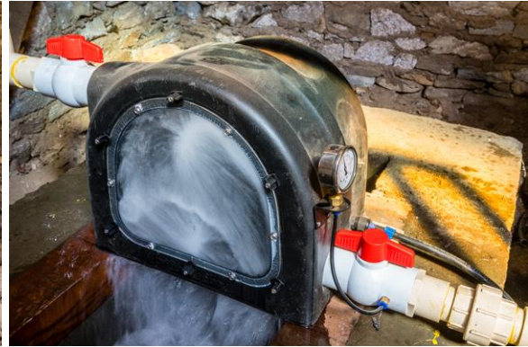
Fig 6: PowerSpout PLT-HP Turbine
