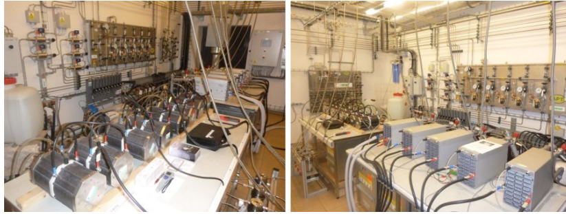
Fig. 3: Fuel cell system (left- electrolyzers, right- fuel cells)
