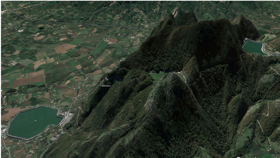
Fig. 1: Example off-river pumped hydro energy storage system at Presenzano, Italy. The upper and lower reservoirs are visible and they are connected via a tunnel. The head is 500 m, the water volume is 6 Gigalitres, the power rating is 1000 Megawatts and the combined reservoir area is about 100 hectares. Image: Google Earth.
