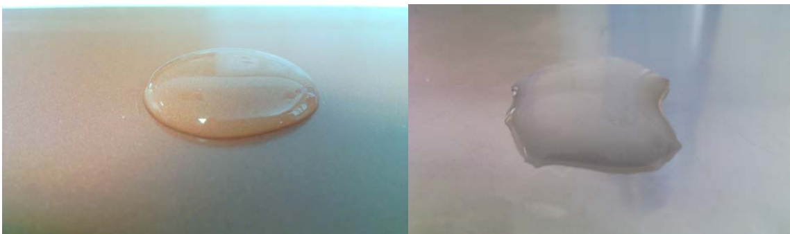
Fig. 3: Water drop on PFA Ruby Red (left) and uncoated steel plate (right).
