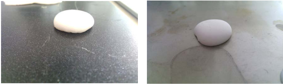
Fig. 4: Crystallized salt drop on ChemCoat (left) and uncoated steel plate (right).
