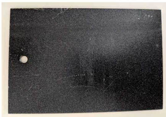
Fig. 11: ChemCoat 1501F. Sliding track below the upper edge visible.
