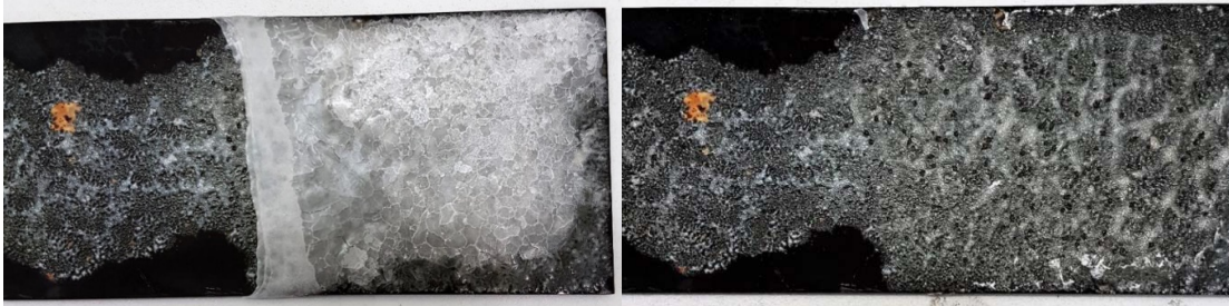
Fig. 2: Sample with Polyox Borosilicate glass coating with an applied layer of Sodium nitrate (left) and after salt was removed (right). (Patsoh, 2017)
