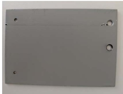
Fig. 10: PFA 7152. Sliding track just below the upper bore holes, damage of the coating on the left side and on the right bore hole of the sliding track.
