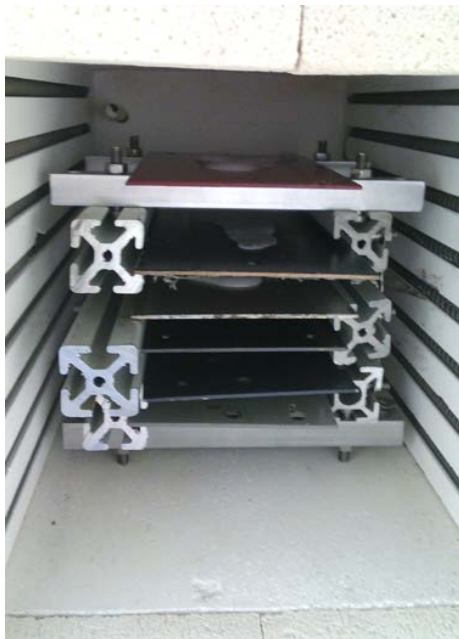
Fig. 5: Testing plates in the oven, wetted with molten salt.
