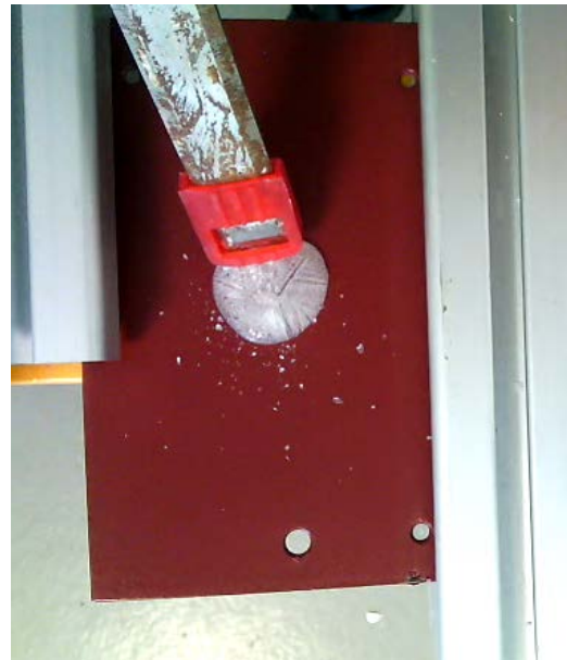
Fig. 6: Test to remove crystallized salt from Ruby Red with hammer and chisel
