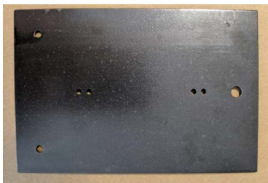
Fig. 13: Durapek, hardly damaged, sliding track slightly visible.
