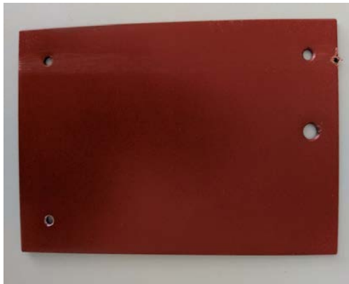
Fig. 9: PFA Ruby Red. Sliding track just below the upper bore holes, damage of the coating on the right side of the sliding track.
