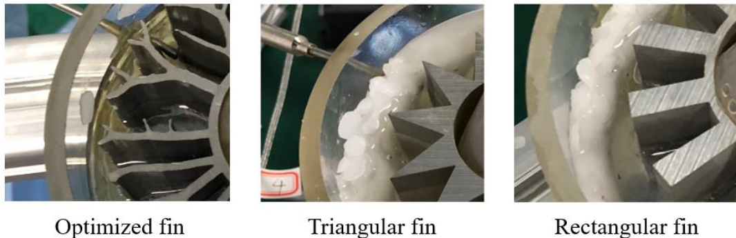
Fig. 10: Comparison of liquid fraction of PCMs with different fin configurations
