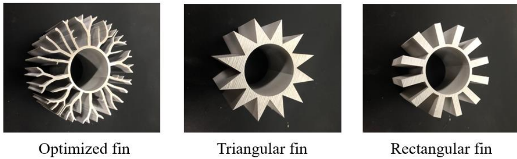
Fig. 3: Three kinds of fin configurations adopted in the experiment
