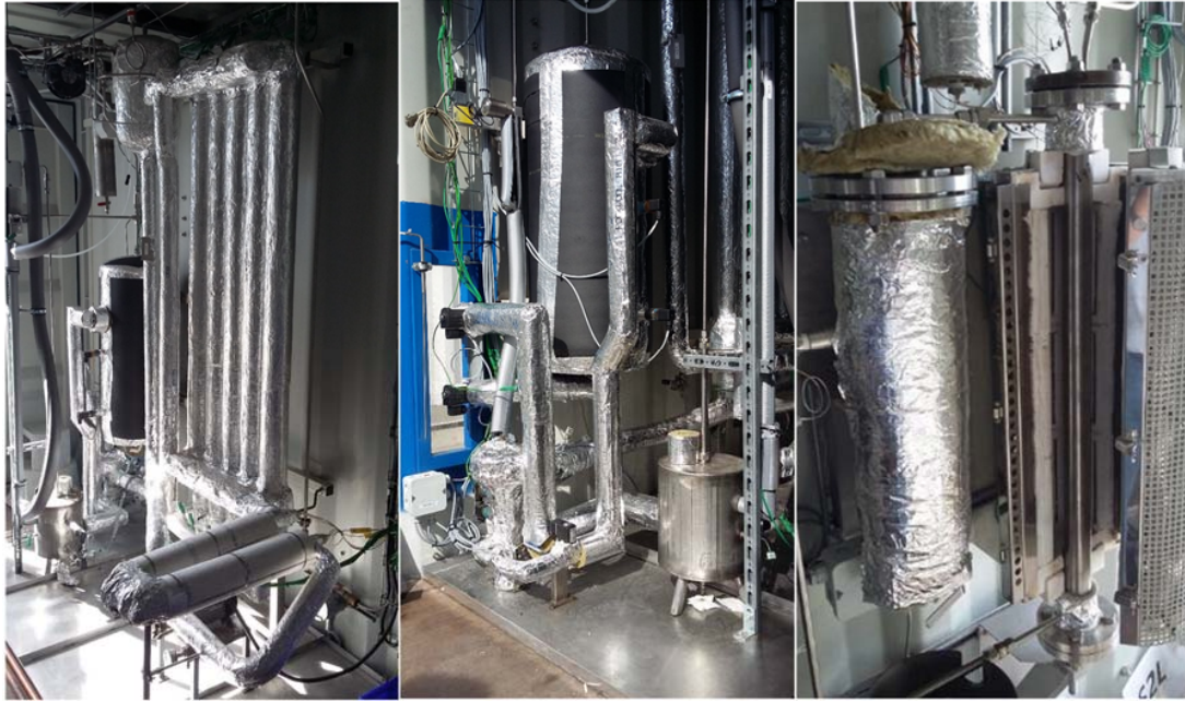
Fig. 10: Main conversion modules in the SUN-to-LIQUID GtL container. Left to right: Fischer-Tropsch reactor tubes, product separation vessel, steam reformer (in opened position) to recycle gaseous hydrocarbons into syngas.
