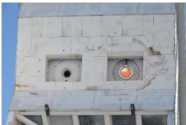
Fig. 14: Right- Solar reactor emitting radiation during oxidation step and cooling down. Left – Calorimetric analogue of solar reactor for confirmation of incident power during testing.
