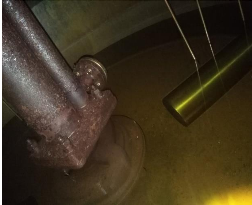
Fig. 3: Ternary mixture composed by 30% LiNO 3 +57% KNO 3 + 13%NaNO 3 inside the tank at 190 ° C during 24 hours without recirculation.
