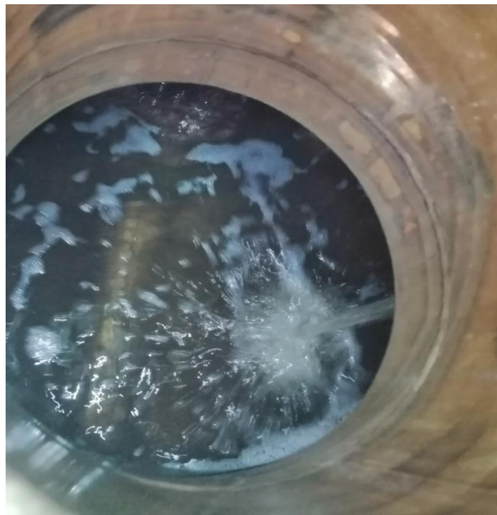
Fig. 4: Recirculation of the ternary mixture in liquid phase inside the sales tank of the pilot plant at 190 ° C after 200 h.
