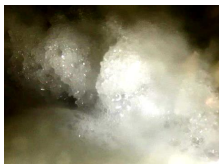
Fig. 2: CO 2 hydrate formed in a pressure vessel (Wang 2016b)
