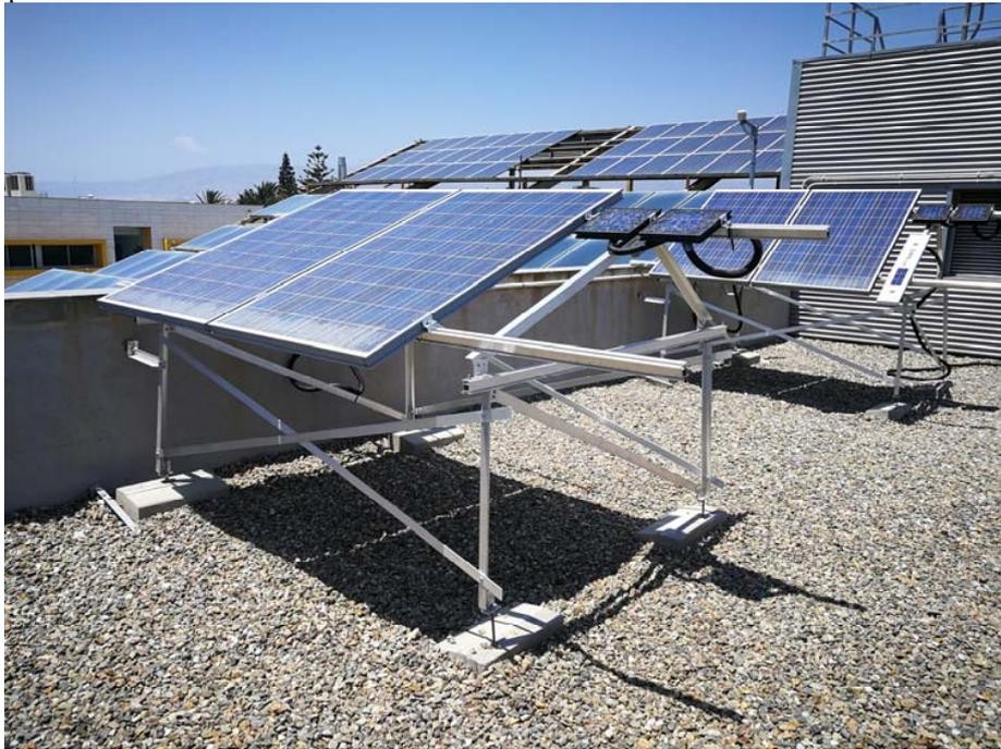
**Figure 13.- PV array together with two calibrated cells.**
