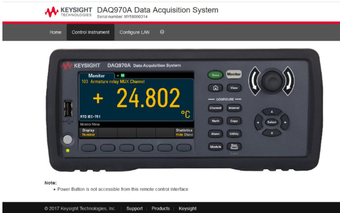
Figure 15.- Interface Web of Datalogger system.
