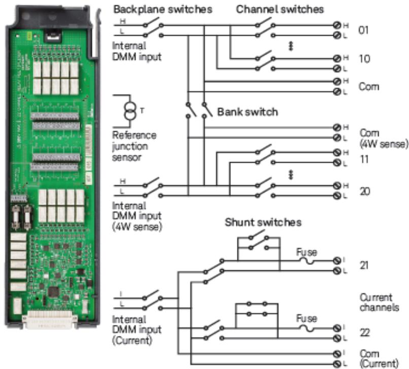
Figure 10.- Internal circuit of DAQM901A.
