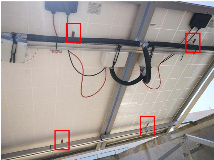
**Figure 14.- Rear view of photovoltaic panels with the identification of the Pt100 sensors.**
