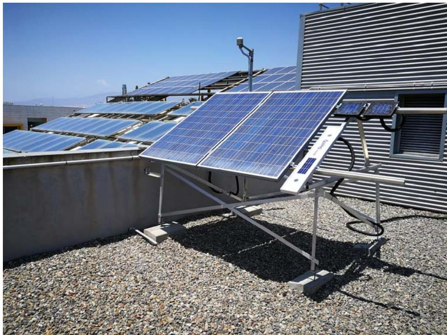
Figure 12.- PV array, DustIQ, calibrated cells and Temperature/HR sensor.
