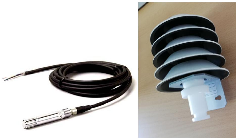
Figure 6.- HMP60 sensor and protection cupule.
