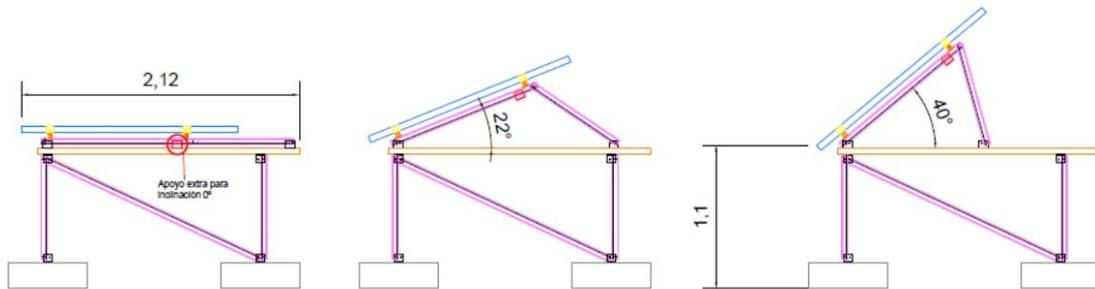
Figure 8.- Plane for the PV panel support structure.
