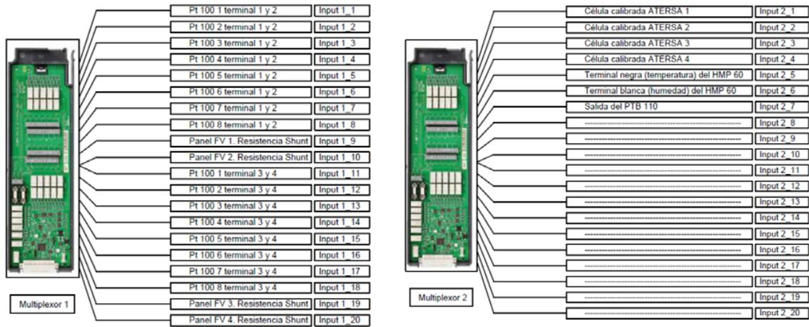
Figure 11.- Connection of sensors in multiplexers 1 and 2.
