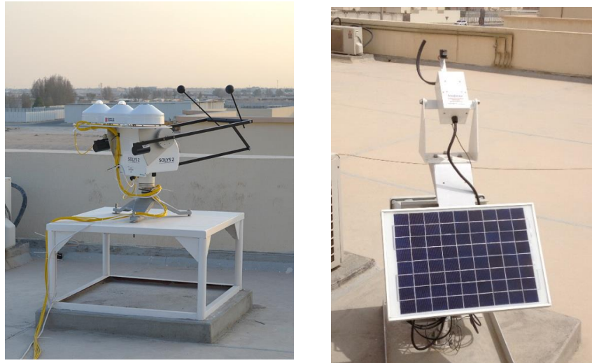
Fig.1: Solar monitoring stations operating in Education City, Doha, Qatar.
