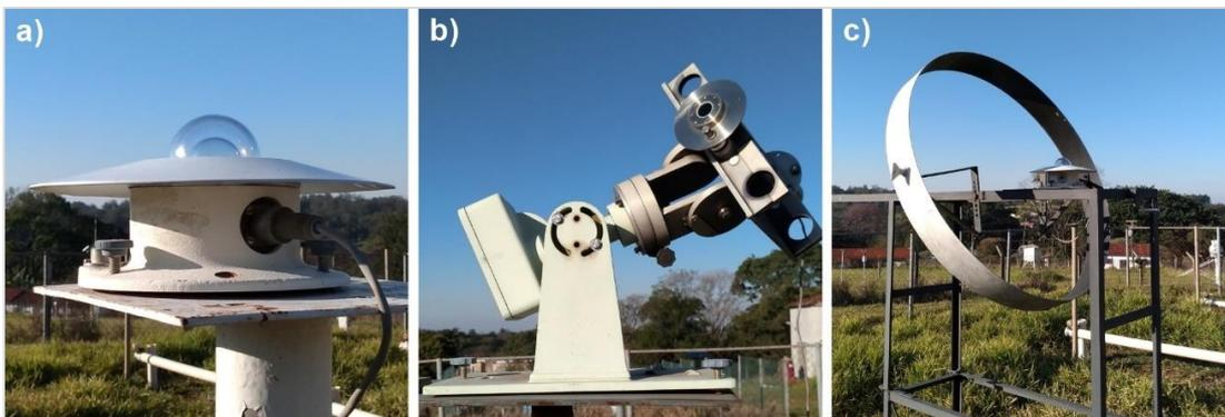
Fig. 2: Pyranometer of global irradiance (a), pyrheliometer of direct-beam irradiance (b) and pyranometer of sky-diffuse irradiance (c) with a shadowring.
