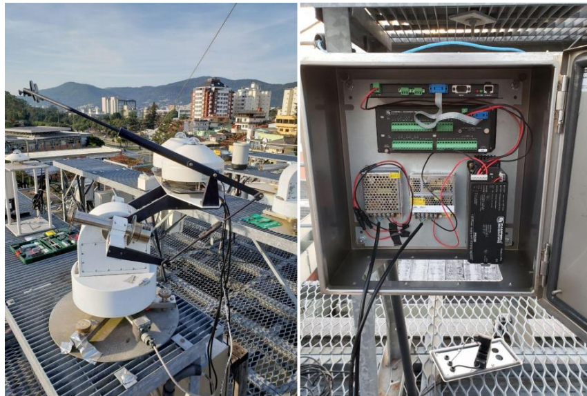
Fig. 6: Instruments and data acquisition system of the solar station.
