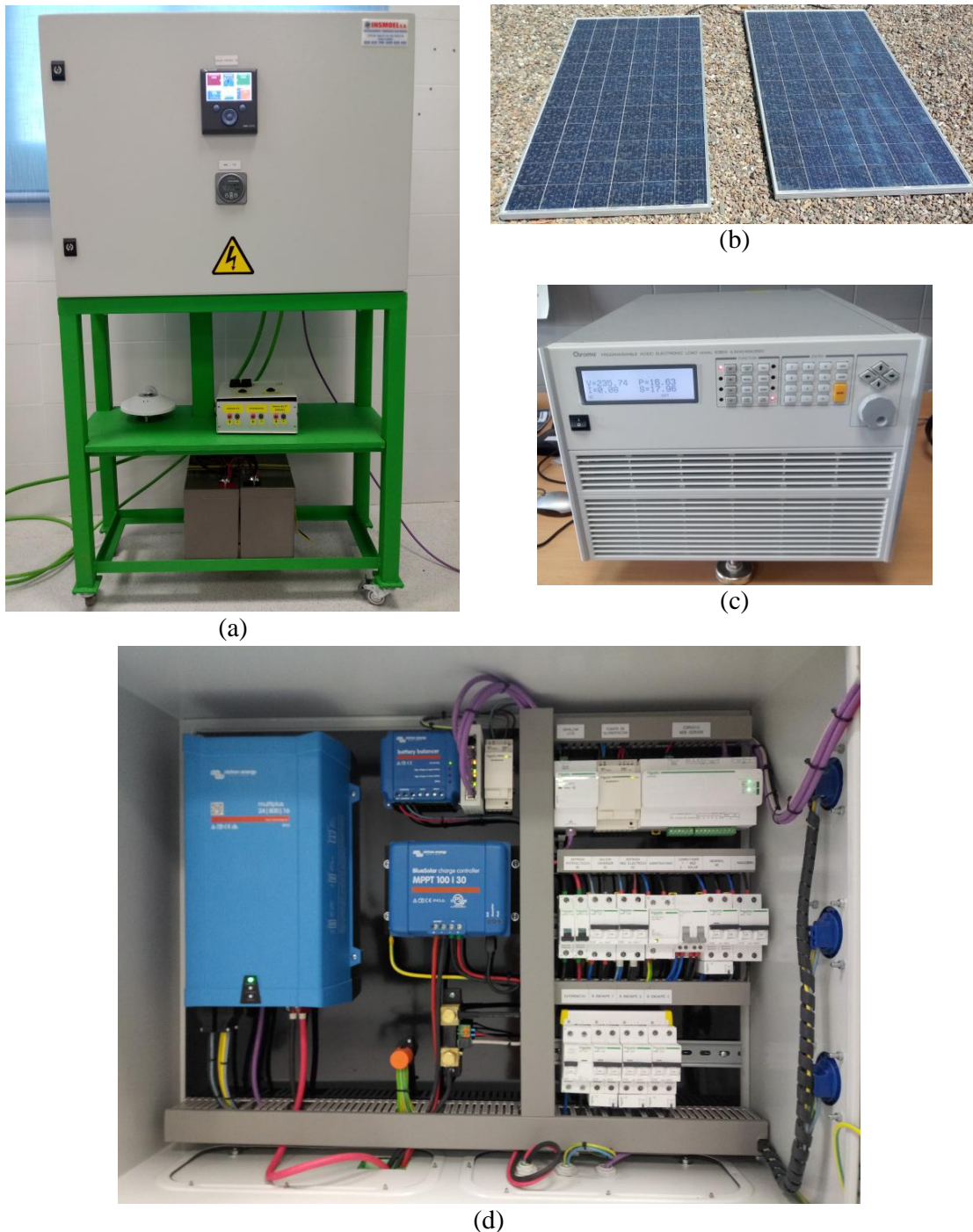
Figure 2. Class material. (a) Batteries and equipment box outer view. (b) Solar panels. (c) Electronic load (d) Box inner view displaying devices setup.
