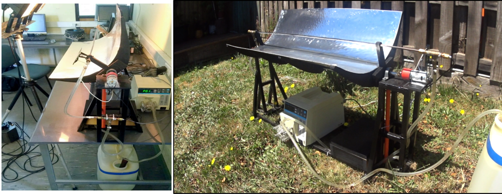
Fig. 3: Parabolic concentrator in the lab (left) and in the field (right)
