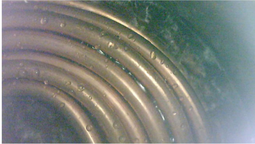
Fig. 6: Droplets on the evaporation/condensing heat exchanger
