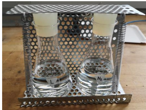
Fig. 3: Erlenmeyer flasks filled with TEG and sealed with silicone plugs including safety mechanism, before starting the high-temperature test. Sample “L” contains air, sample “N 2 ” is passivated with Nitrogen.
