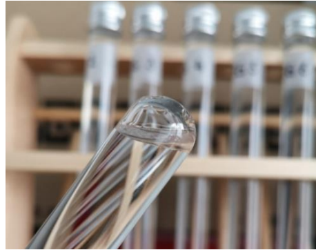
Fig. 2: Test tube filled with TEG and remaining air bubble (foreground) and further test tubes prepared for long-term UV exposure test (background)
