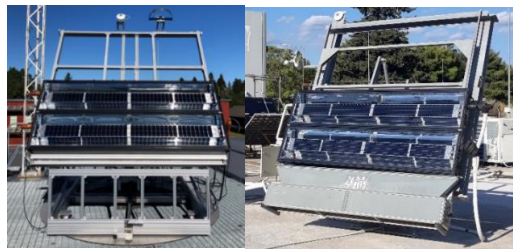
Figure 3. CPVT solar collector test apparatus is located in the Solar Laboratory of the University of Gävle (left image) and at NCSR D (right image).
