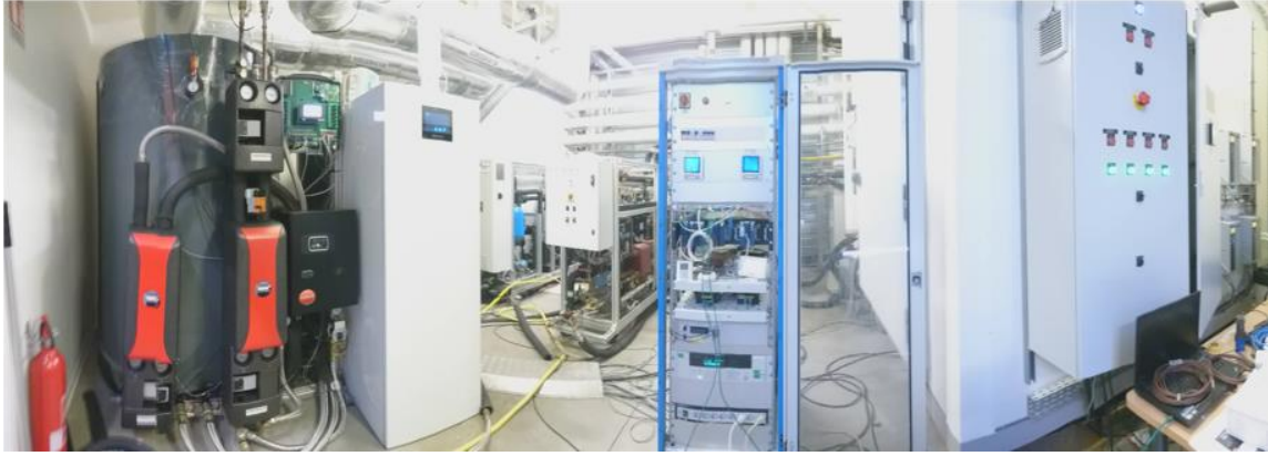
Fig. 4: HS2 concept and outlook of real prototype integrated in semi-virtual test bench
