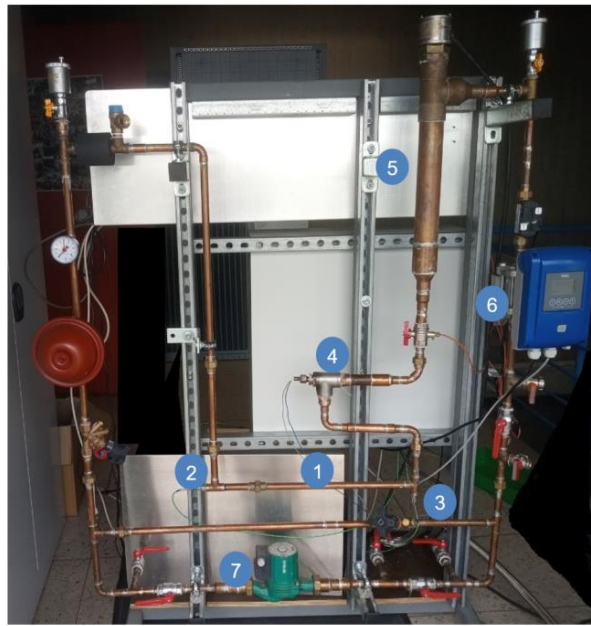
Fig. 7: Measurement test rig to generate actual temperature profiles as of the hydraulic loops of the thermal system
