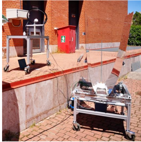
Fig. 5. Pyranometer's installation (left) and the CPC prototype used (right).
