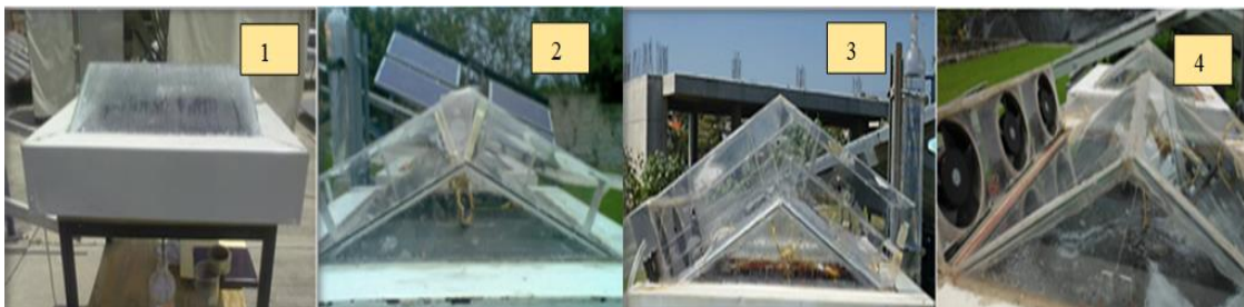
Fig. 1: DSSS in operation: 1) Natural convection, 2) Natural convection with acrylic cover, 3) Forced convection, fans in serial and double slope, 4) Forced convection, fans in serial and without wind tunnel
