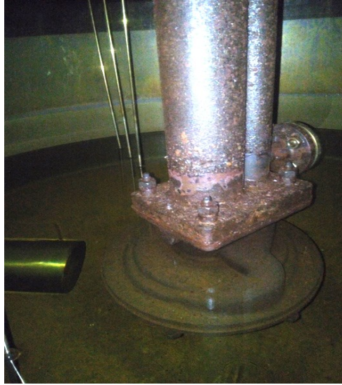
Fig. 2: Cooling of the ternary mixture with 30% LiNO 3 + 57% KNO 3 + 13% NaNO 3 inside the tank at a temperature of 190°C.
