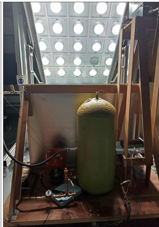
Fig.2: Solar thermal system on a test rig
