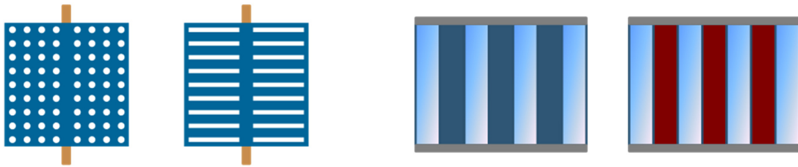
Fig. 4: Perforated absorber sheets to increase the daylight supply (left); Façade design options with colored absorbers and alternating arrangement of transparent, conventional and opaque, solar-active U-shaped profiled glass (right)
