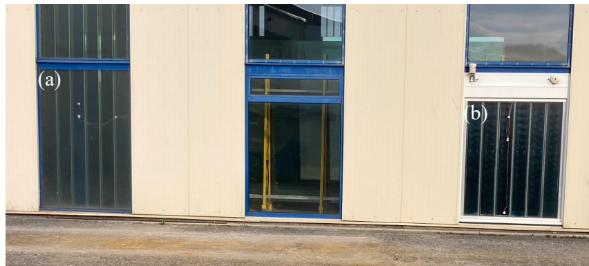
Fig. 8: Façade-integrated, solar-activated profiled glass module (b) and reference profiled glass module (a), with sensors for recording the temperatures and hemispherical radiation (glass surface and absorber temperature placed at 2/3 of the aperture height)
