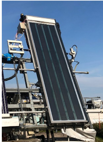
Fig. 7: Large test façade module during the measurement on the sun tracker at ISFH ( 4 \text{ m} \times 1 \text{ m} )
