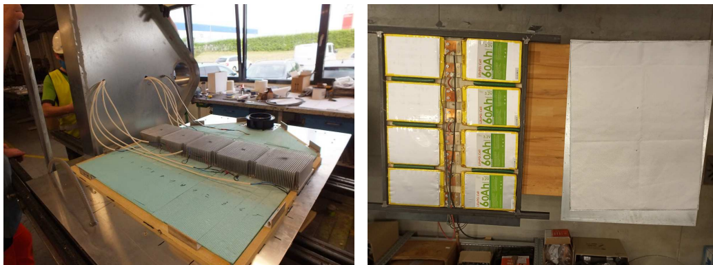
Fig. 2: Peltier AC unit with finned heat sinks (left), flat-plate battery layout (right)
