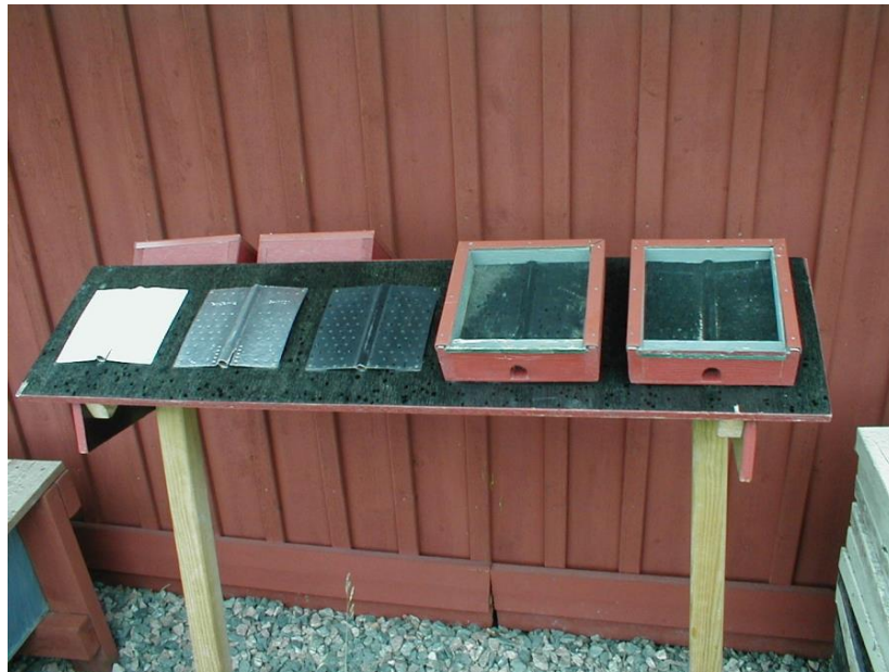
Fig.5. Solar Surfaces Demonstrated at Teknoland. Exhibit label: Feel the different surface temperatures! A black surface absorbs more sunlight than a white or a metallic. A surface turned towards the sun than one that is turned away from the sun. Glazing prevents radiation from the surface. A painted surface radiates heat easier than a metal surface and is therefore cooler.
