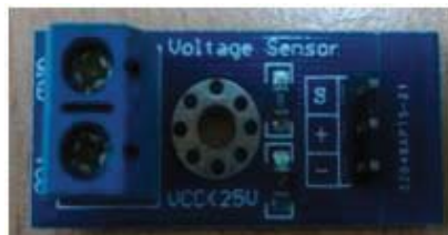
Fig. 5: Voltage sensor and connection diagram to arduino
