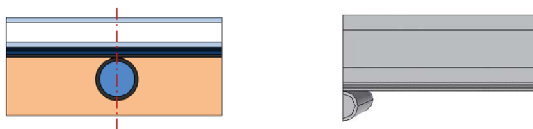
Fig. 2. (Left) Cross section of a pipe and its fin and (right) half a pipe modelled in COMSOL Multiphysics
