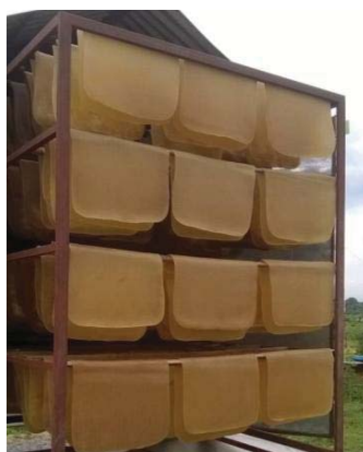
Fig. 10: The features of rubber after drying for three days in solar drying chamber
