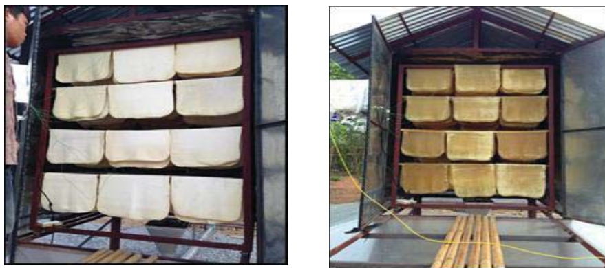
Fig. 9: Features of the rubber sheets (a) before and (b) after 2 days of drying.
