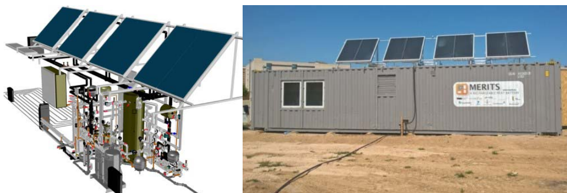
Fig. 1: MERITS Field Test Demonstrator 3D systems model (left) and Field Test Demonstration container during pre-testing in Lleida, Spain (right)
