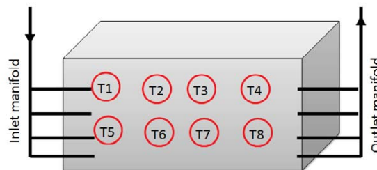
Figure 3: Schematic of the thermocouples position inside the compact heat storage.
