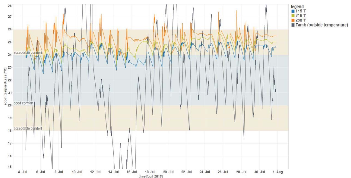
Fig. 11: Room temperatures in July 2016 between 07:00 and 18:00
