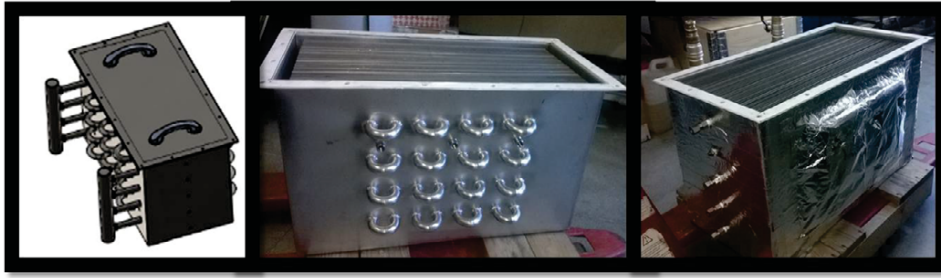
Figure 2: the fin-and-tube heat exchanger for the latent storage, 3D rendering and pictures of the system before and after thermal insulation.
