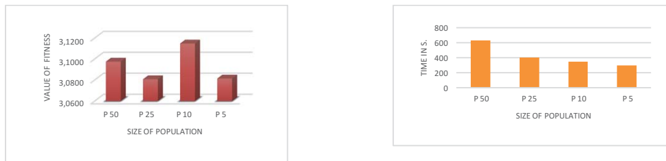
Fig. 10 Effect of the population size: a) value of the fitness function b) time spent
