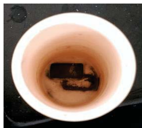
Figure 5: Corrosion observed in 304SS immersed in saline 32%Li 2 CO 3 +35%K 2 CO 3 + 33%Na 2 CO 3 at 650C during 500 hours of test
