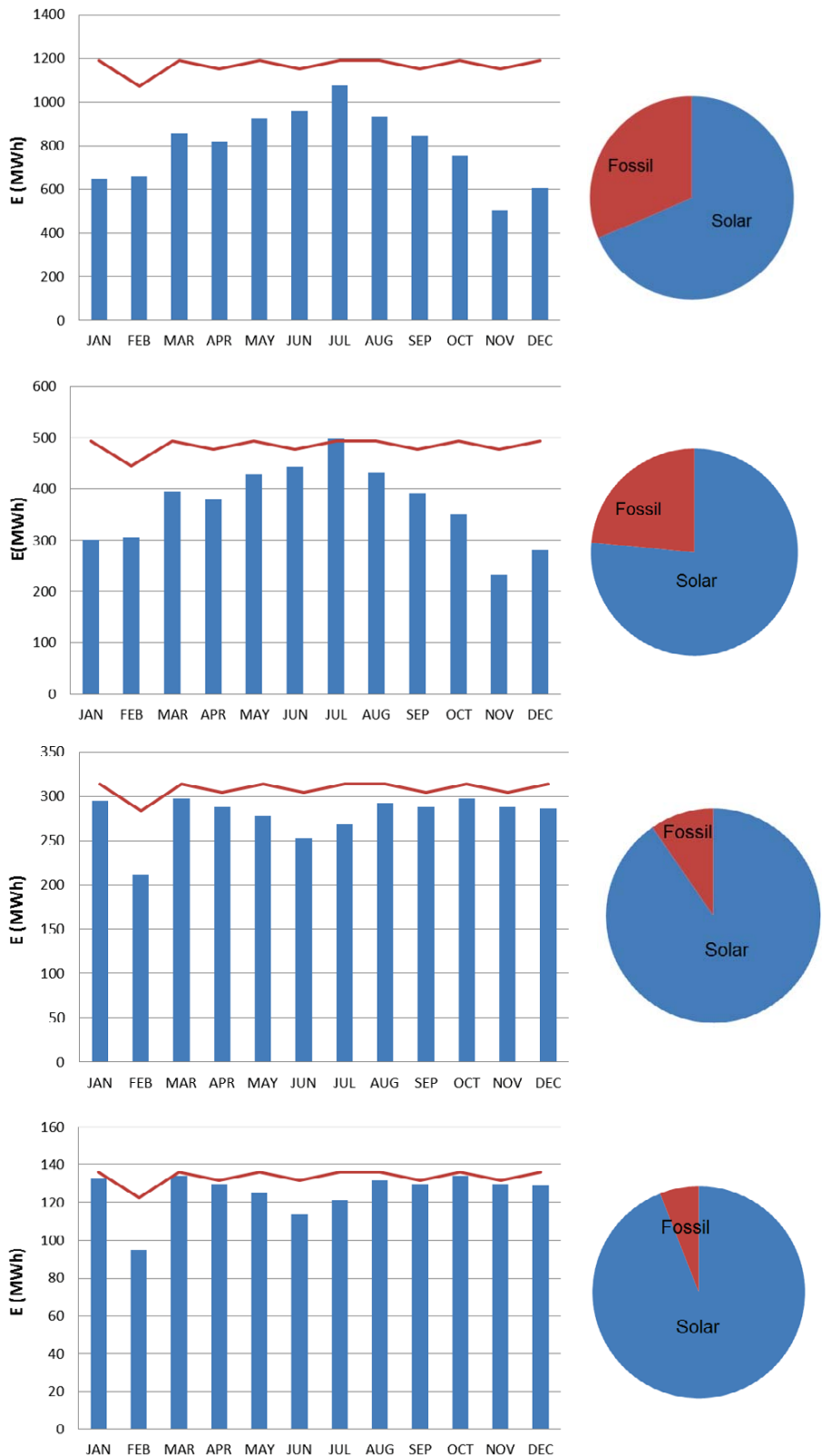
Fig.3. Energy production by the plants dimensioned to the cases described in section 5 per month during a typical year (case 1, 2, 3 and 4 respectively). Red line indicates the monthly heat demand. Fraction of the heat demand that should be provided by conventional fuels, according to the proposed designs.
