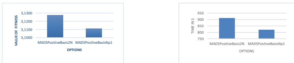
Fig. 9 Effect of PollMethod parameter: a) value of the fitness function b) time spent
