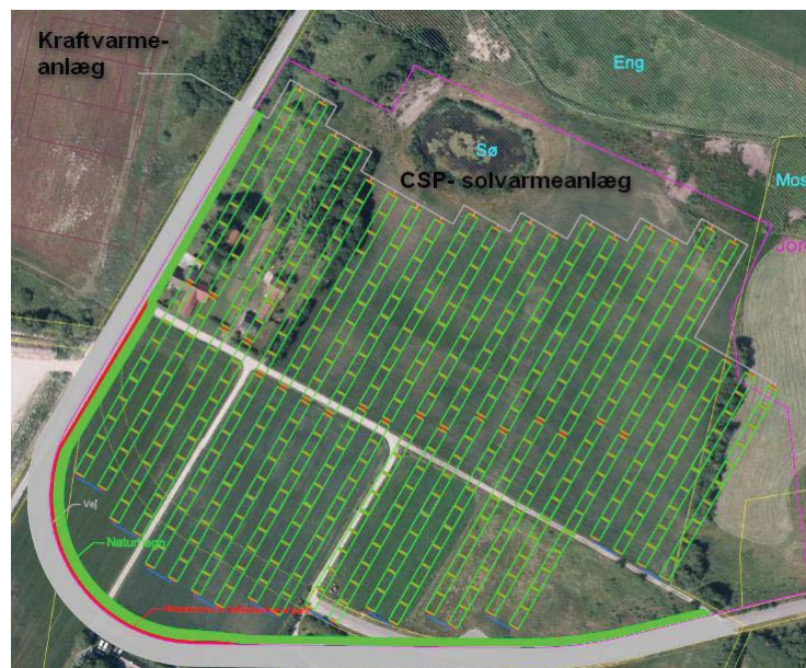
Fig 5. Photo of the 27000 m 2 CSP collector field with row layout in Brønderslev. Note that the troughs are turned approximately 30 degrees from south to match the available land area. This has been found to reduce the annual performance relatively little and was a finding in [2] giving a large flexibility in installation of such plants.
