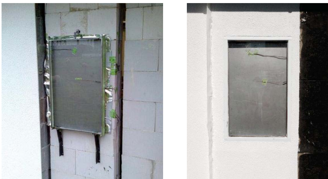
Figure 2: STI demonstrator with dimensions 80 cm x 50 cm, installed at a massive test façade. Left figure: Real STI demonstrator setup without surrounding insulation and plaster. Right figure: Real STI demonstrator setup after thermal insulating (black coloured) and plastering (white coloured).
