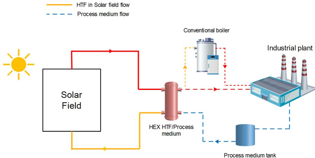
Fig. 1: Integration of solar heat in an existing industrial plant
