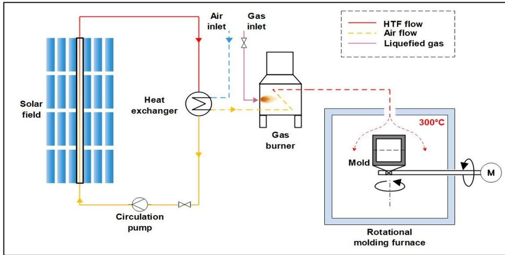
Fig. 4: scheme of the proposed solar heat integration in RMP
