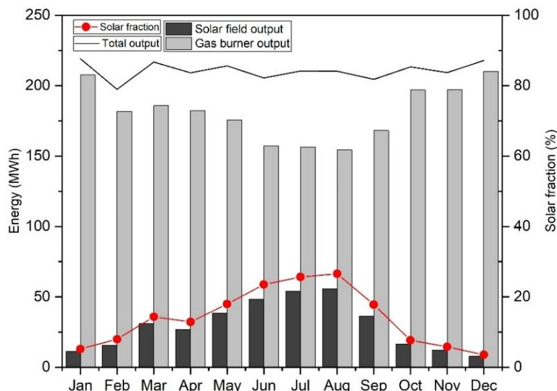
Fig. 8: Monthly solar fraction for the optimal configuration
