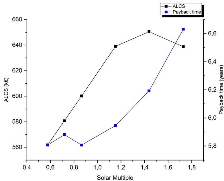
Fig. 7: ALCS and payback time with respect to SM
