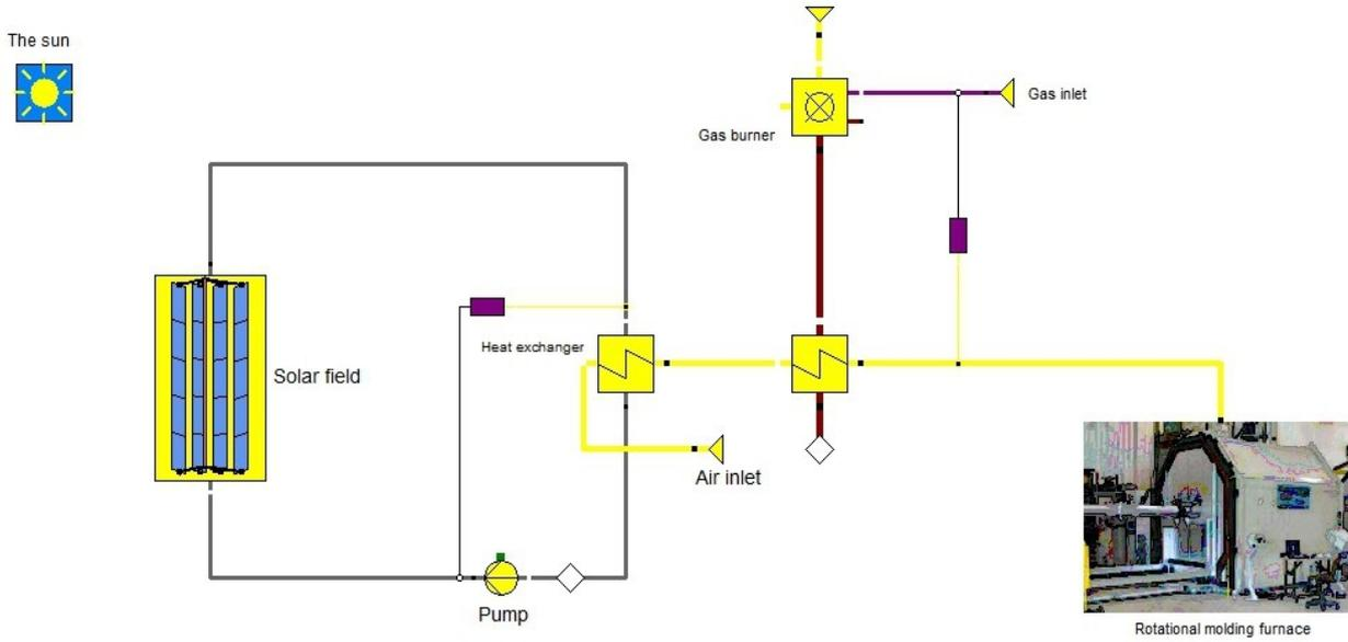
Fig. 6: Layout of the proposed model in EBSILON
