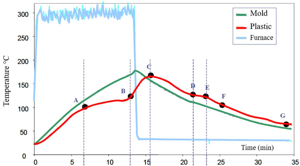
Fig. 3: Temperature variation during a rotational molding cycle (Pérot, 2006)
