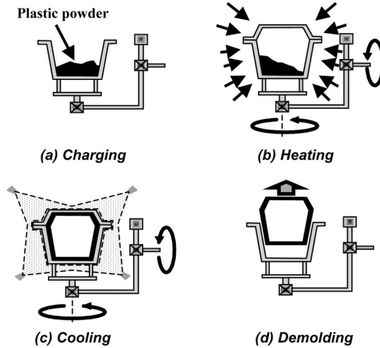
Fig. 2: Steps of rotational molding process (Crawford et al., 2002)
