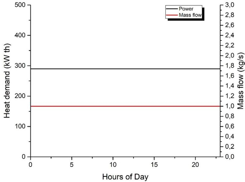
Fig. 5: Heat demand profile of the process
