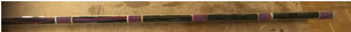
Fig. 1: Glass tube with temperature sensors (T1-T5) for temperature measurements inside the tank
