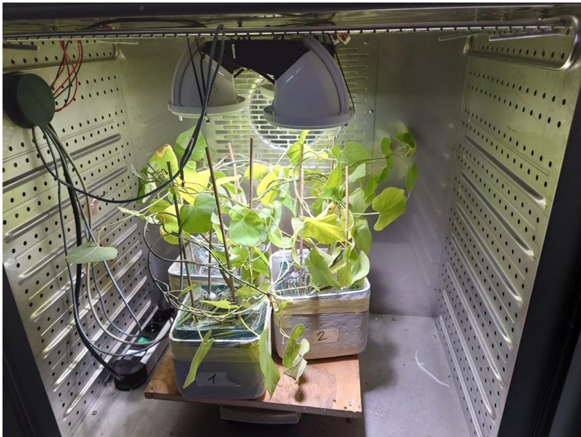
Fig. 1: Measurement setup in the climate chamber to determine the transpiration of different plants. The plants were placed on a scale and illuminated with three lamps, whose spectrum is specially designed for plants, type DL2 from RVG LICHT.
