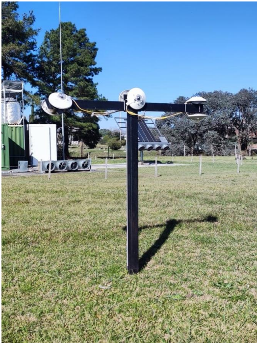
Fig. 1a: Albedo measurement setup, including G_h and G_g sensors (both instruments on the right; the others are for inclined solar irradiance, not used in this study).
