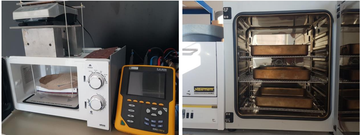
Fig. 1: Multimode fixed-bed microwave oven with balance and power-meter (left), conventional hot-air drying oven (right)
