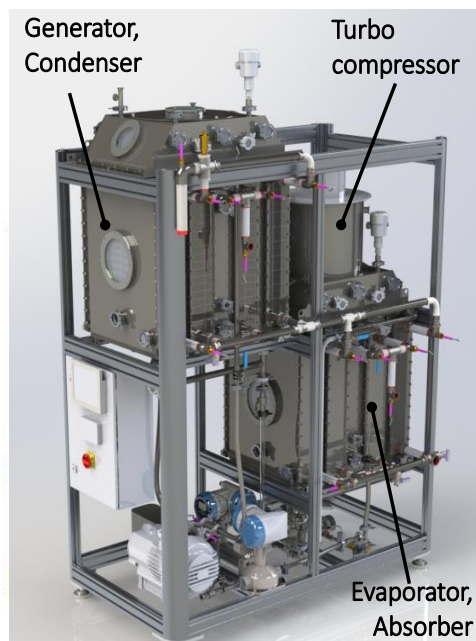
Figure 1: Design of the lab-scale hybrid chiller (Schweigler, 2019).
