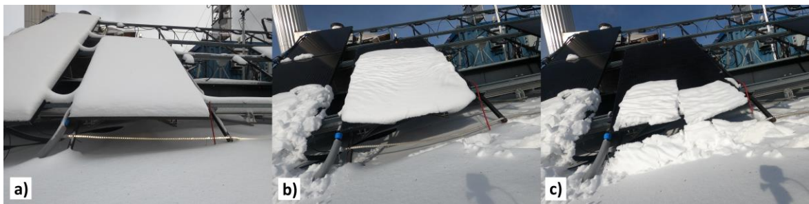
Fig. 8: Snow shedding process on the front side of the finned panel showing a) full snow cover, b) shedding start, and c) shedding end.
