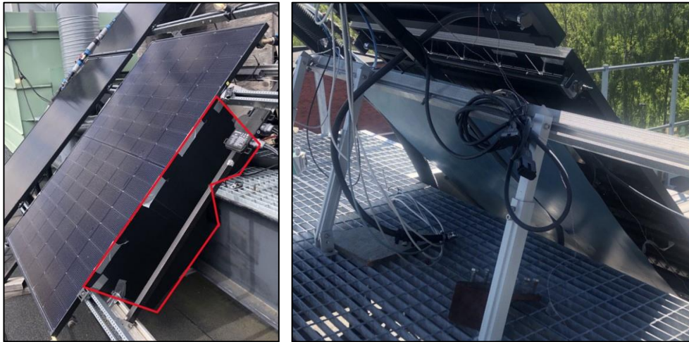
Fig. 4: Left) Side panels attached behind the PV panel. Right) Back panel attached 14.5 cm behind the absorber of the PVT.
