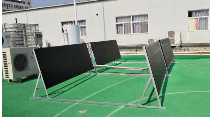
Fig. 6: Prototype of the solar and air dual-source heat pump water heater system
