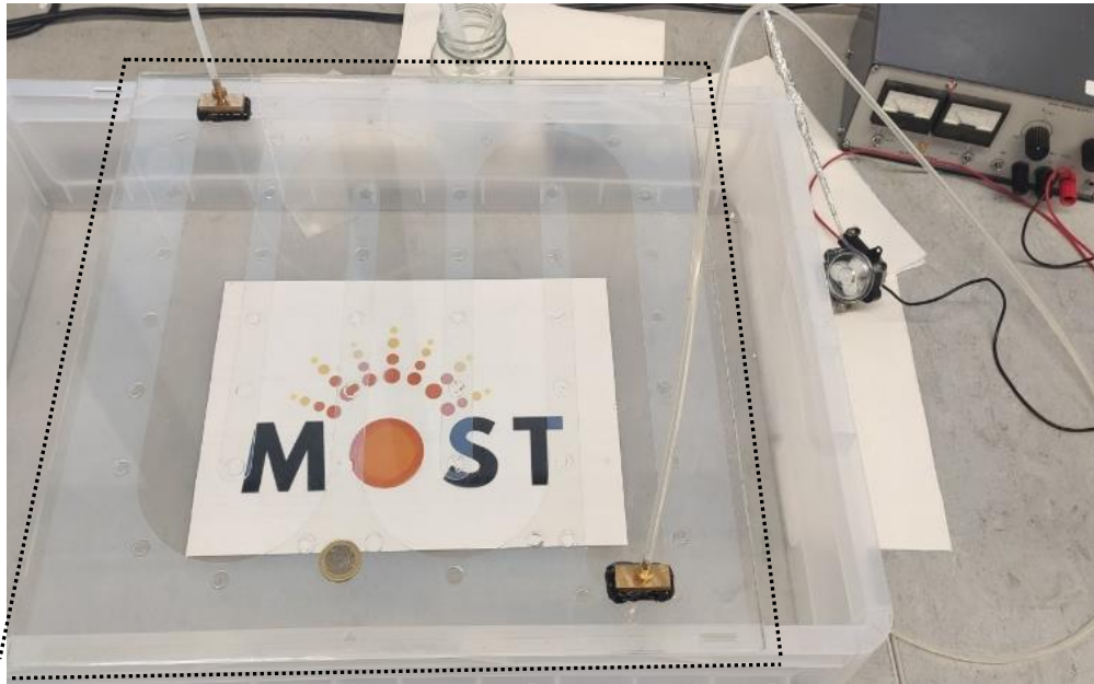
Figure 11: Almost fully transparent thermal oil resistant collector with DELO PHOTOBOND GB368. For better visibility, the edges of the collector are marked with a dotted line.
