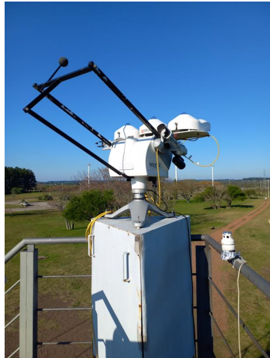
Fig. 1b: SOLYS2 system with G_d and G_b sensors.
