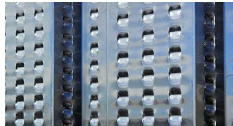
Fig. 1: Closeup of perforated aluminum selective surface.
