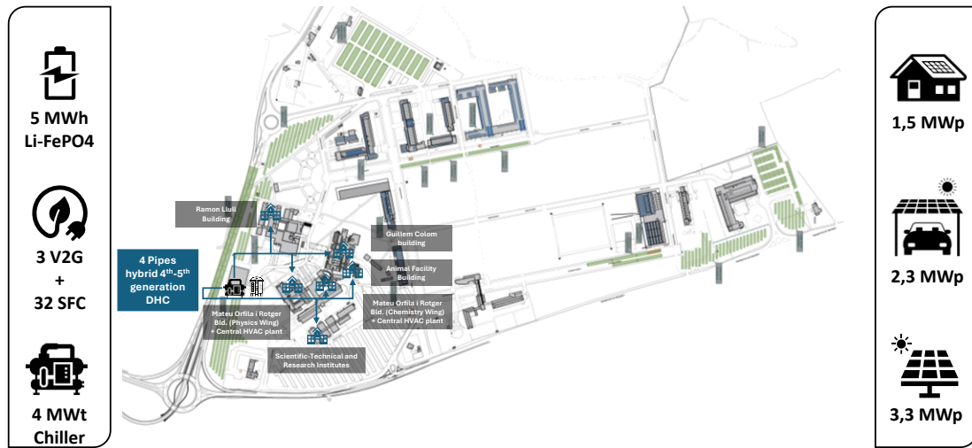
Fig. 1: Distribution of the renewable generation plants to be deployed at the UIB campus, located in Palma de Mallorca, Spain
