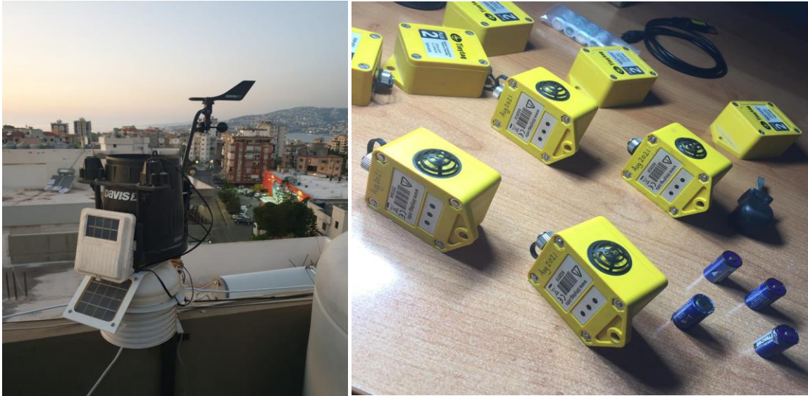
Fig. 3: Photos showing the instruments used for dry bulb data collection. Source: Author on August 2023.
