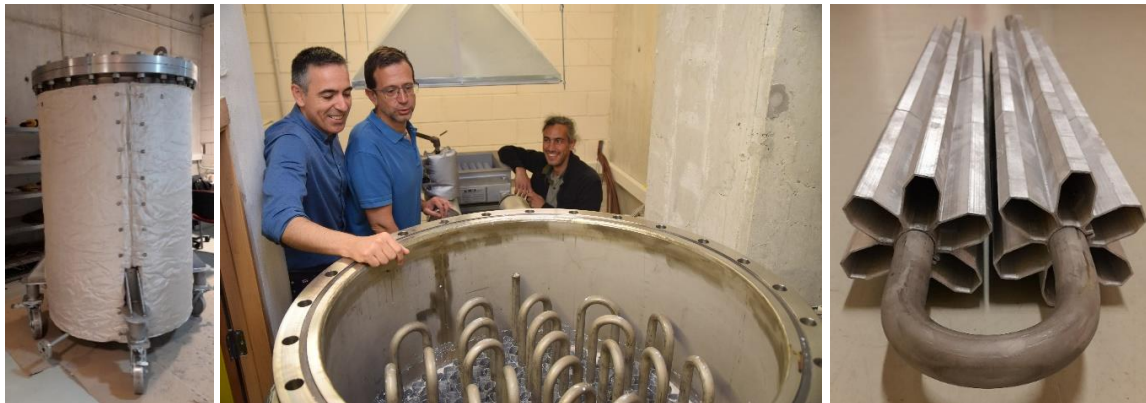
Fig. 9: Accumulator of the storage system and detail of the inserts
