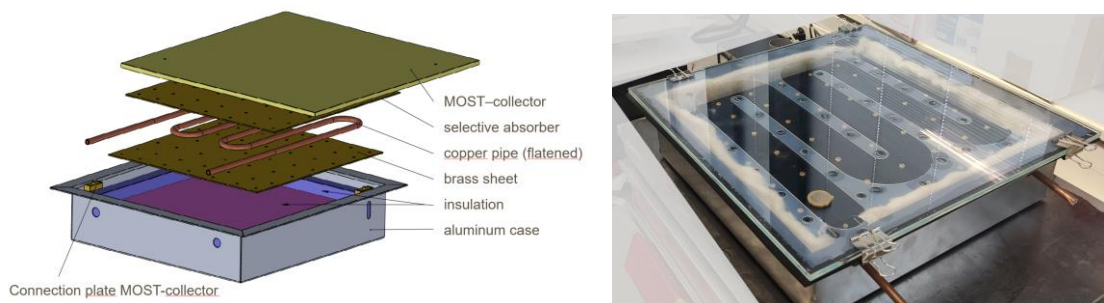
Figure 12: Left: Exploded view drawing of the first hybrid collector (MOST collector (top) + solar thermal collector (below)); right: Picture of the finished hybrid collector.
