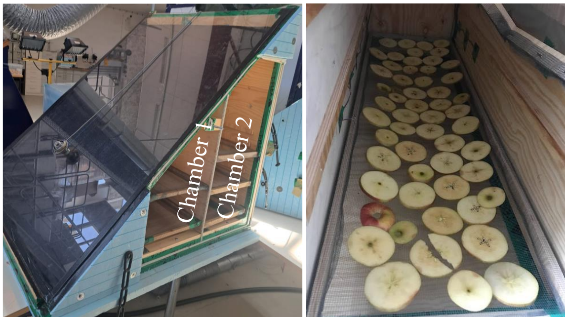
Fig. 2: Left: Photo of the solar dryer. The two chambers are indicated in the photo. Right: Photo showing the placement of apples on the trays.
