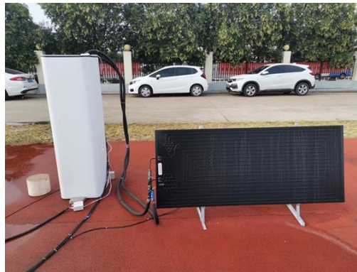
Fig. 4: Prototype of the solar direct-expansion heat pump water heater system
