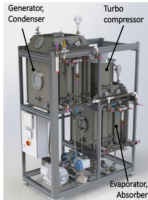
Figure 1: Design of the lab-scale hybrid chiller (Schweigler, 2019).
