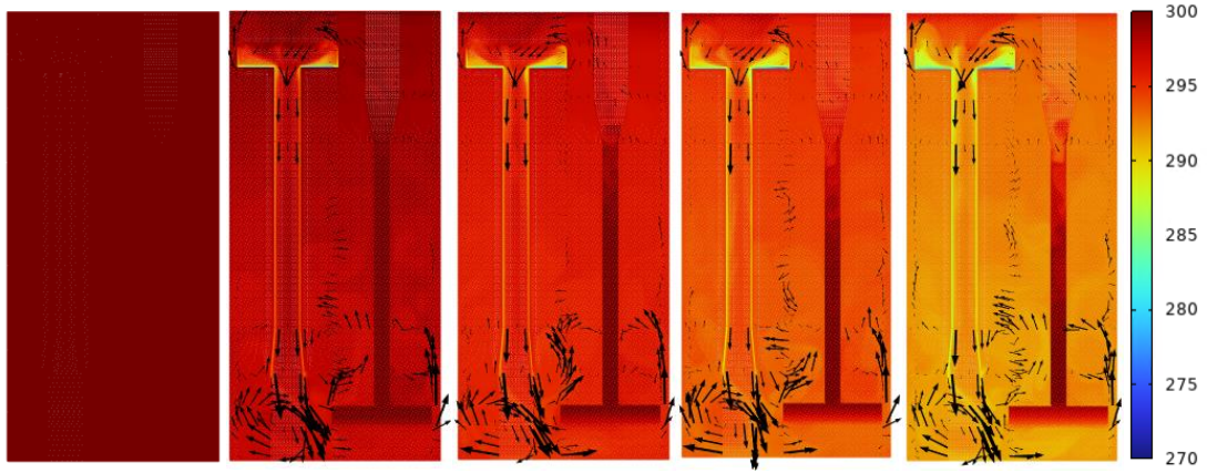
Fig. 2: Temperature ( ^{\circ}\text{C} ) distribution and flow direction in the tank for different times during discharge (heat sink of 1 \text{ MW m}^{-3} and no momentum sink in the heat exchanger).
