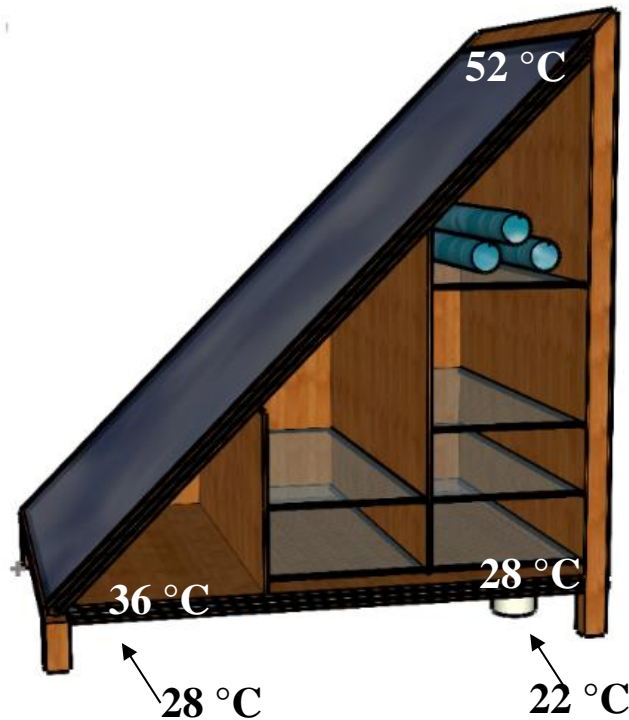
Fig. 8: Temperature distribution in the dryer.
