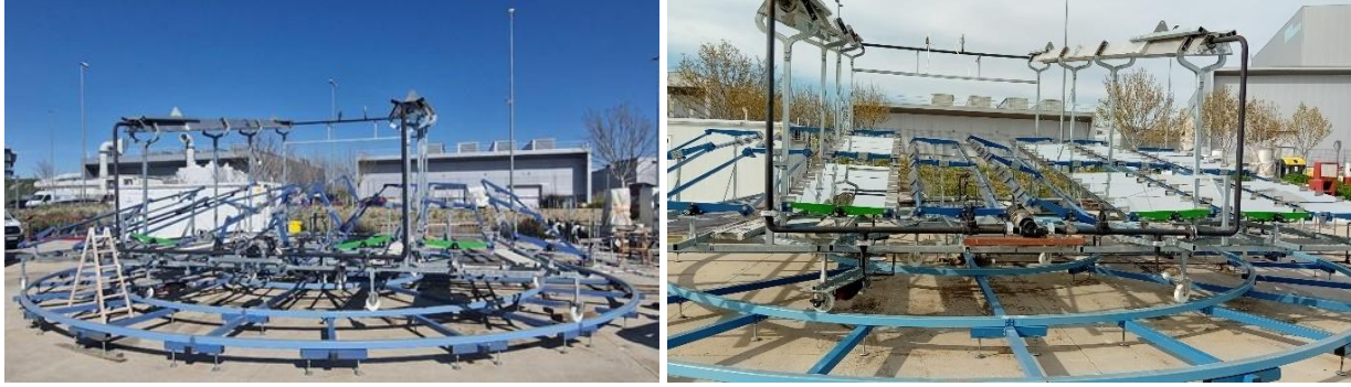
Fig. 7: SunDial with single axis tracking system for the Mandrekas case study, before (left) and after (right) placing the reflectors
