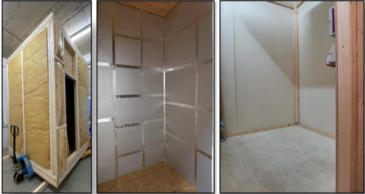
Figure 6: Pictures of the thermally high insulated test chamber. Left: Outside of the chamber with 100 mm mineral wool. Middle: 20 mm vacuum insulation panels installed to the inside of the chamber. Right: Inner top layer of 12 mm multiplex board.
