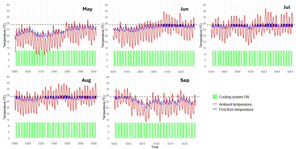
Fig 8. Thermal evolution in the first floor over the simulations months. The green line indicates when the cooling systems can operate.
