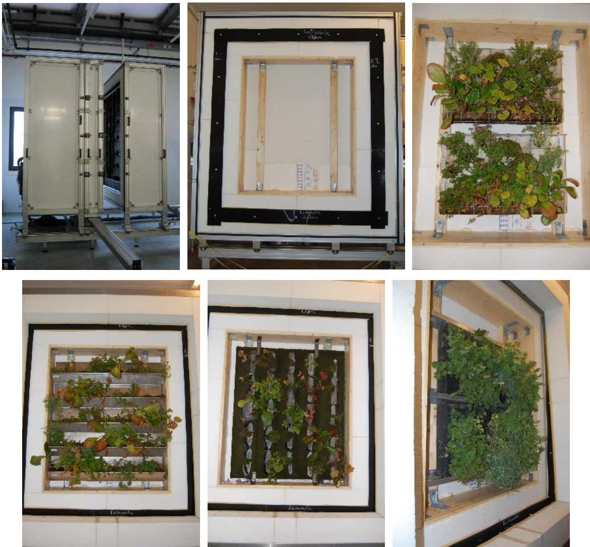
Fig. 1: Hot-Box system (top left), reference wall (top mid), and LWS samples: gabion system (top right), tray system (bottom left), modular system 1 (bottom mid), and modular system 2 (bottom right).
