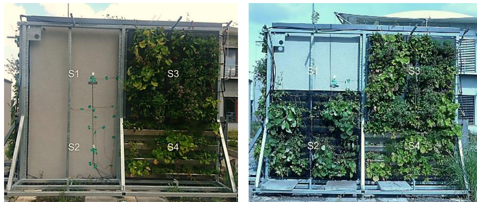
Fig. 3: South façade with two different LWS at the beginning of the measurement period on July 20, 2023 (left) and after the measurement period on September 20, 2023 (right). In the right picture, there's already a new system installed on S2 for the winter measurements; this was not measured during summer.
