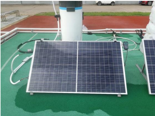
Fig. 8: Prototype of the PVT heat pump water heater system
