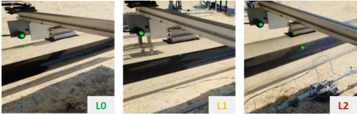
Figure 3. Experimental setup for measuring transmittance of the parabolic trough receiver over the experimental campaign.
