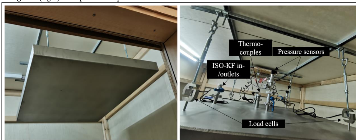
Figure 4: Photo documentation of the evaporator. Left: The evaporator installed as cooling ceiling into the test chamber. Right: View on the top of the evaporator with sensors.
