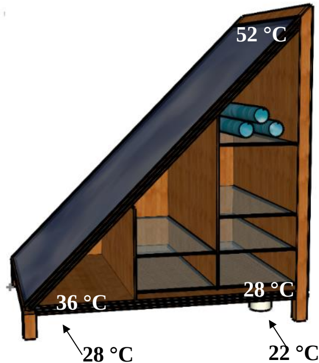
Fig. 8: Temperature distribution in the dryer.
