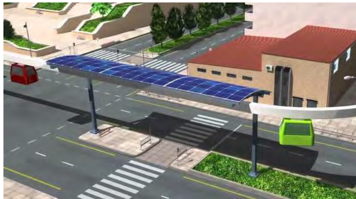
Figure 1: Solar Powered Automated Transit (ATN). Relatively small vehicles traverse a network of exclusive guideways and utilize off-line stations to provide on-demand, non-stop, origin-to-destination mobility. Suspending the ATN vehicle below the guideway makes the upper surface available for PV panels that can power the system. (Jpods system, from (Wilmott, 2015)).
