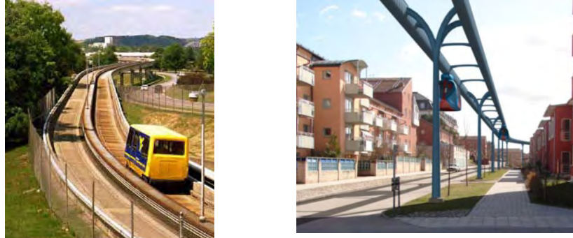
Figure 3: Supported vs. Suspended ATN vehicles. The Morgantown PRT on the left is a ‘supported’ system, where vehicles ride on top of the guideway and are supported by it. The Beamways system on the right depicts a suspended system where the vehicle hangs beneath the guideway. (Morgantown photo from http://www.progressiveengineer.com/PEWebBackissues2002/PEWeb%2024%20Mar%2002-2/24photos/PRT1.jpg . Suspended vehicle rendering from Beamways, http://www.beamways.com/wp-content/uploads/beamways_system_en.pdf )
