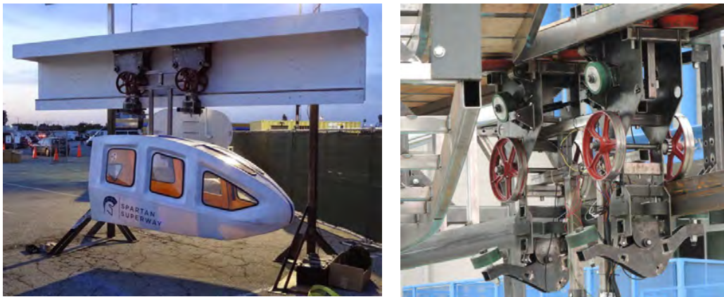
Figure 4: Full-scale demonstration models of the Superway guideway and bogie. The photo on the left (from Maker Faire 2014) shows the bogie supporting a mock (not full-scale) vehicle on a short length of straight guideway. The photo on the right shows the bogie and steering mechanisms on a section of guideway that includes a ‘Y’ switching section. The model on the right, from the exhibit shown at Maker Faire in 2015, demonstrated the steering mechanism and the ability for the bogie to navigate both directions of the ‘Y’.
