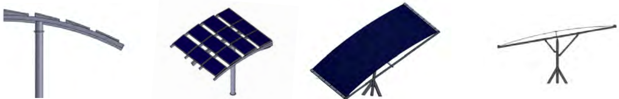
Fig. 10: Initial concepts design of the mounting array for the solar panel modules
