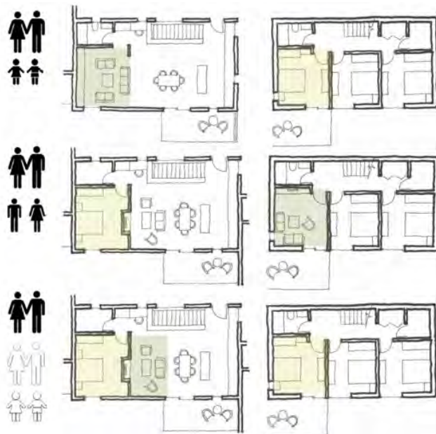
Fig. 4: Variations and Adaptability in Floor Plans Image Source: Penn State 2014-2015 “Heritage Homes” Race to Zero competition team.
