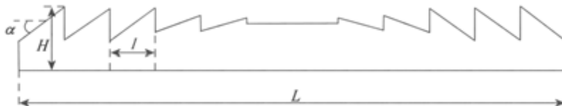
Fig. 2- The secondary optics is a cylindrical Fresnel lens with this profile.
