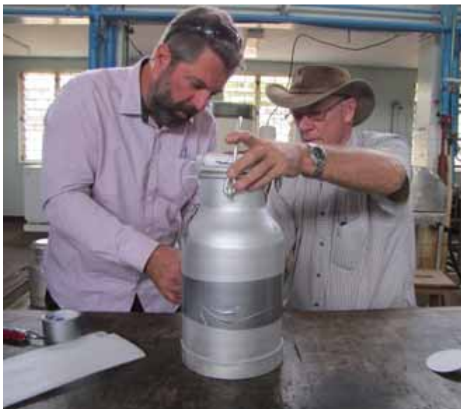
Fig. 6: Brian Jensen of SDZR and Bruce Knight of WI install a temperature probe and small datalogger on a 10 liter milk can at Egerton University Dairy Lab.
