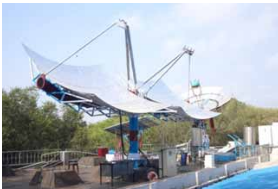
Fig. 4: A prototype of the HCPV system developed for the BioCPV project.
