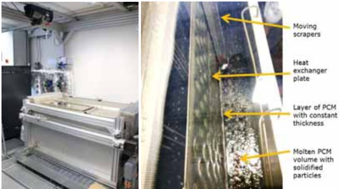
Fig. 2: Test facility with storage unit (left). Storage during commissioning, showing moving scraper that keeps frozen PCM layer at constant thickness (right).
