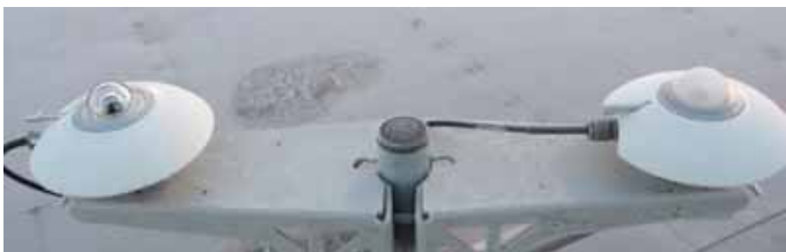
Fig. 5: Visual difference between a heated (left) and unheated (right) pyranometer during frost. Data points measured with the left pyranometer can be assigned a meaningful uncertainty, data points measured with the right pyranometer have to be flagged as not available.
