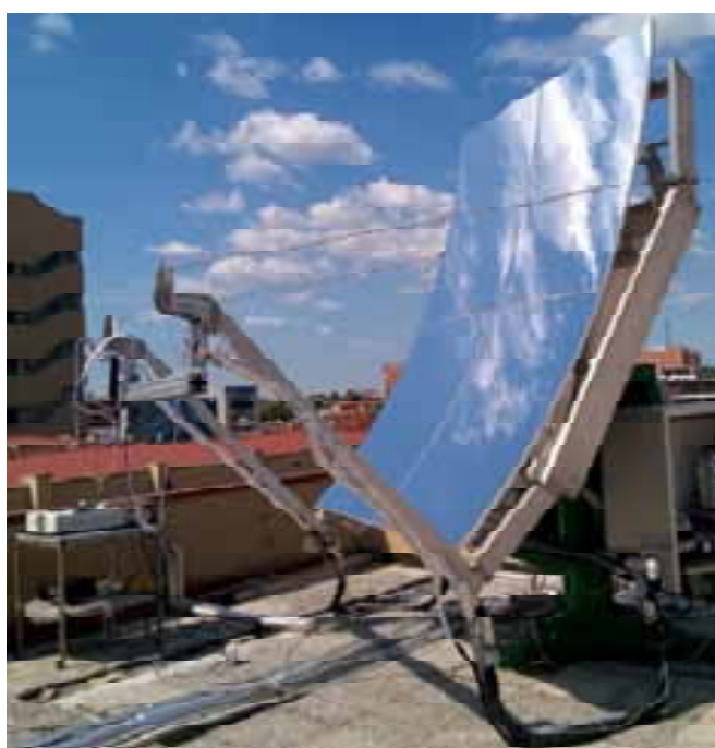
Fig. 1: Prototype of the asymmetrical parabolic trough linear solar concentrator and solar flux map measuring system installed at the Solar Energy Conversion Lab of the University of Padova.
