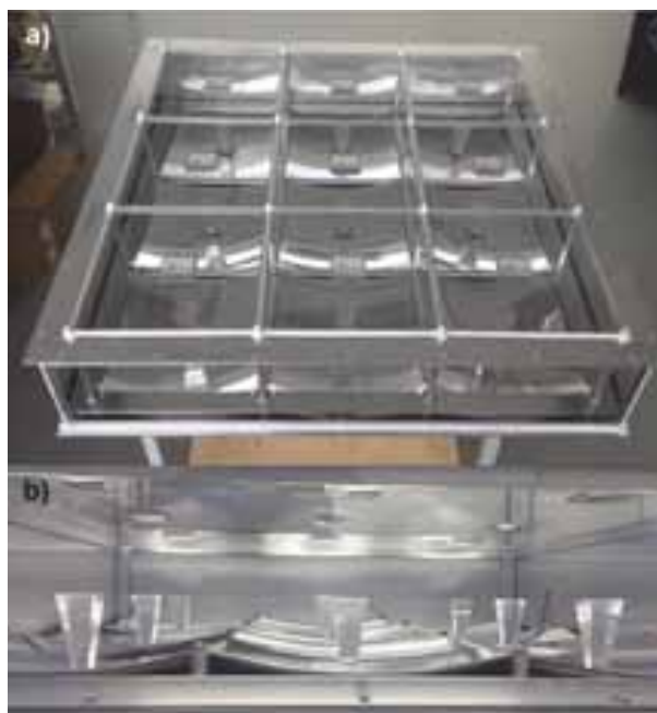
Fig. 7: The 3x3 Cassegrain Concentrator Photovoltaic System a) top and b) side view.
