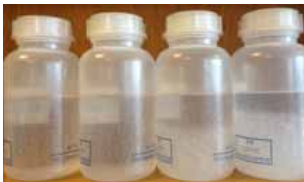
Fig. 6: 8 cm salt water mixtures after 131 days supercooling, 46%, 45%, 42%, 40% water samples from left to right
