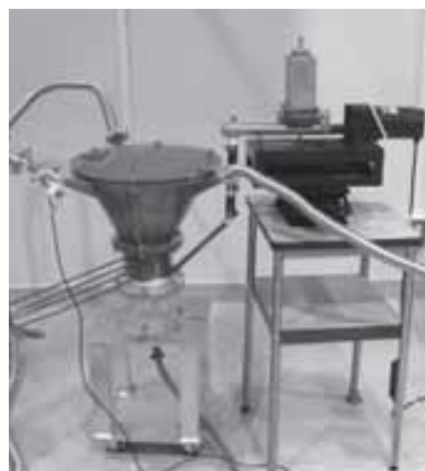
Figure 2 Photograph of experimental system using fluidized bed reactor combined with screw feeder for coal-coke supply.
