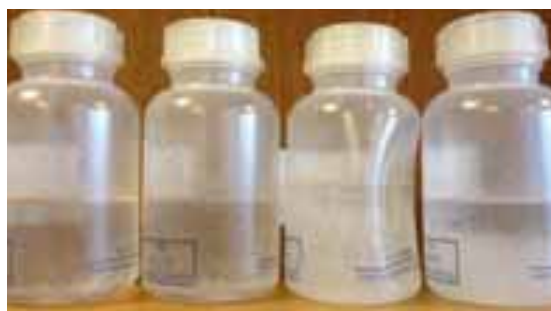
Fig. 4: 4 cm salt water mixtures after 126 days supercooling, 46%, 45%, 42%, 40% water samples from left to right
