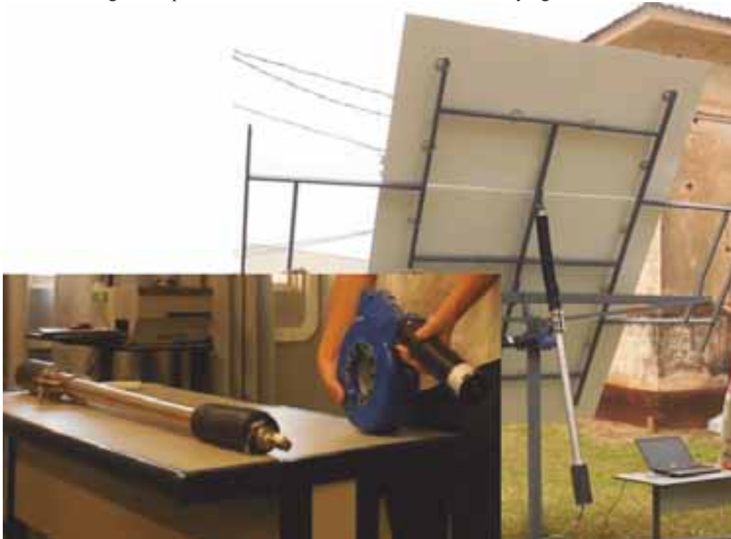
Fig. 1: Drives of a first heliostat design with comparably expensive drives from abroad and too flexible mirror support structure (mirror not complete).
