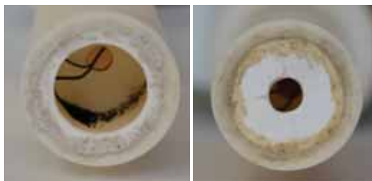
Fig. 3: Ceramics rings. Front ring was changed after first experiments in order to avoid sample losses
