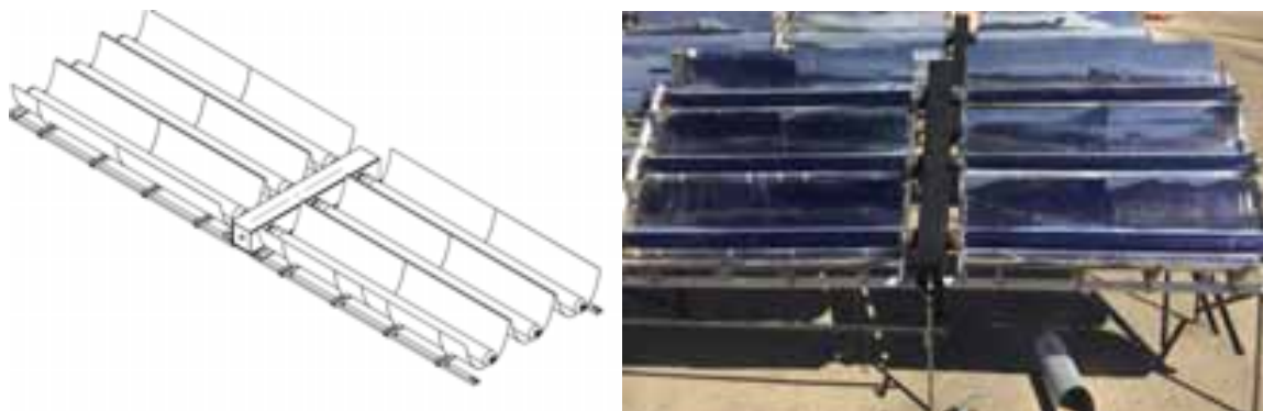
Fig 4: The XCPC collector with east west axis direction. Aperture area for each collector is 4.5 m 2
