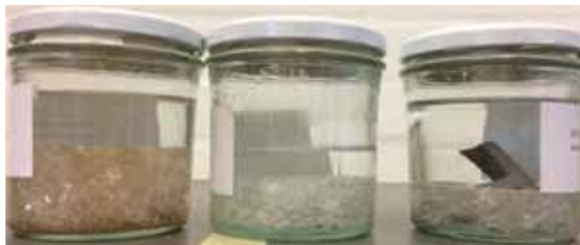
Fig. 1: Long term supercooled sodium acetate trihydrate water mixture samples
