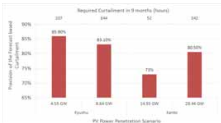
Fig. 4: Precision of required curtailment detection with a forecast based curtailment for Kyushu and Kanto in two PV power penetration scenarios.
