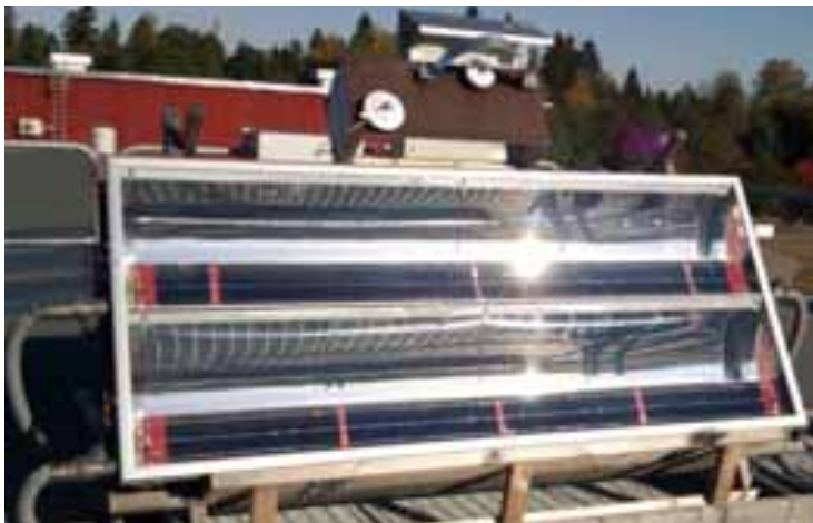
Fig. 1: Solarus C-PVT collector and solar radiation sensor
