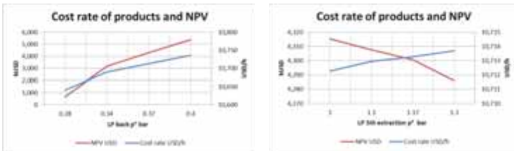
Fig.11: Effects of: a- LP turbine backup pressure, b- LP turbine 5th extraction pressure.
