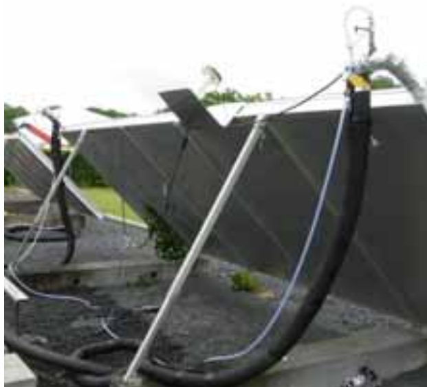
Figure 2: Solar collector HT-SA 35/10 used for the validation and plastic pipes arrangement for pressure drop measurement.
