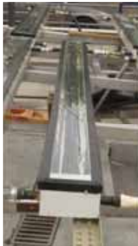
Figure 4: CPC designed and built.
