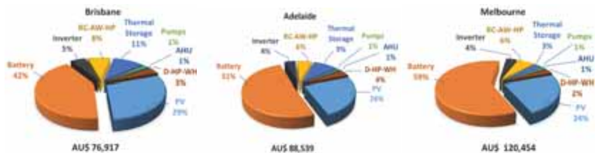
Figure (2) the life cycle cost break down to main forming components in the three climates
