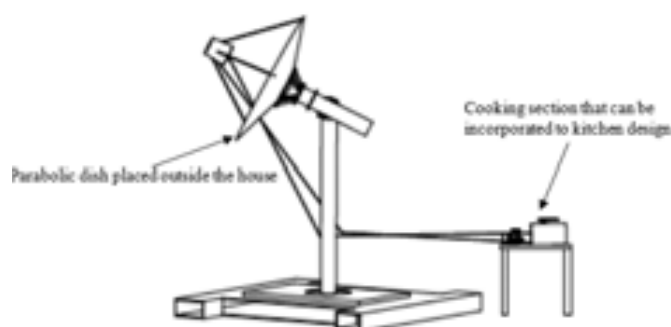
Figure 2: Complete CAD drawing of the experimental setup
