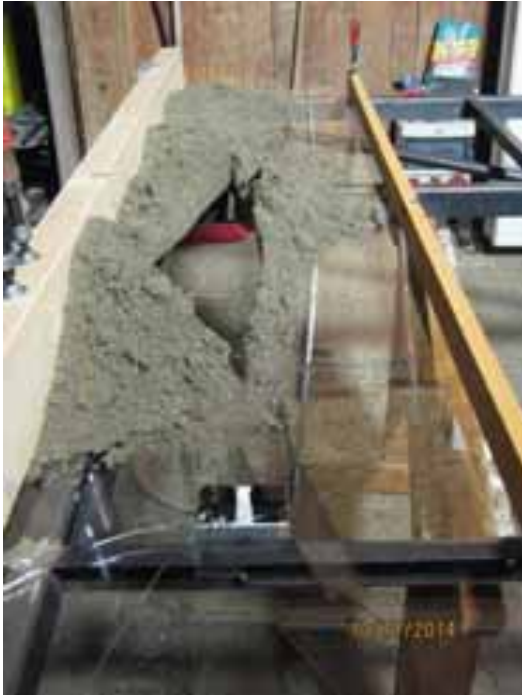
Fig. 13: Breakage of 4mm glass stripe before reaching of maximum expected load.
