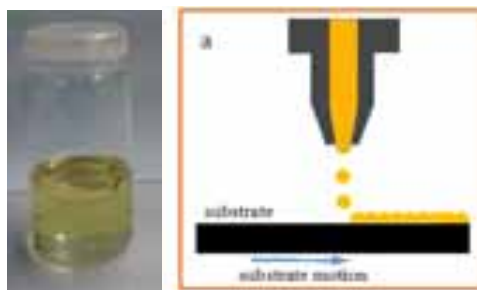
Figure 2: Formulated ink and operation principle of inkjet printing.
