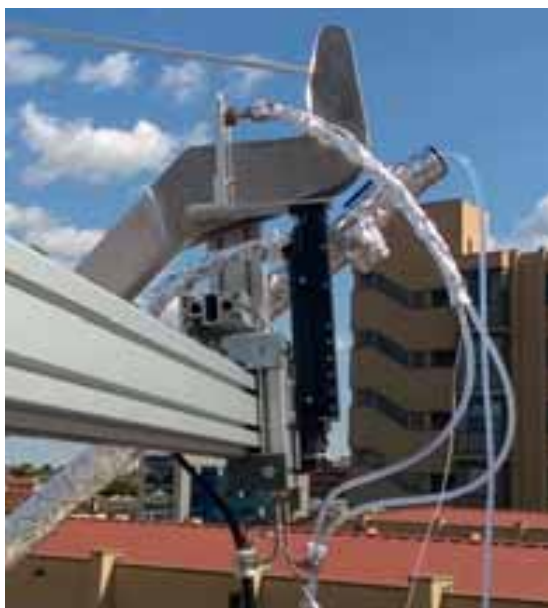
Fig. 2: Electric linear actuator mounted on the sliding carriage of the x-axis and water-cooled heat flux microsensors arranged on a supporting structure.
