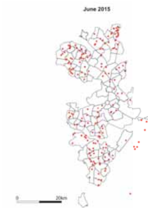
Fig. 1: PV systems in Canberra which are actively reporting their power output every five minutes to PVOutput.org, before being ingested into the Regional PV Simulation System. The black lines are the boundaries of Canberra suburbs
