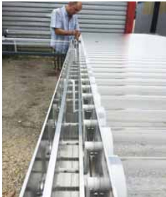
Fig. 7: Rolling mechanism stress tests
