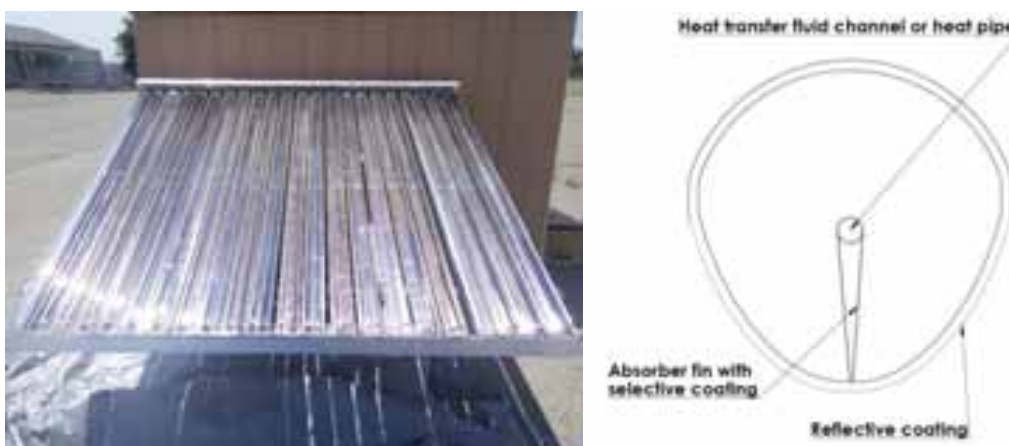
Fig 5: a) The ICPC 3.5 m 2 prototype, with full 1900mm length tube, front view. b) The cross section of the original ICPC prototype design.
