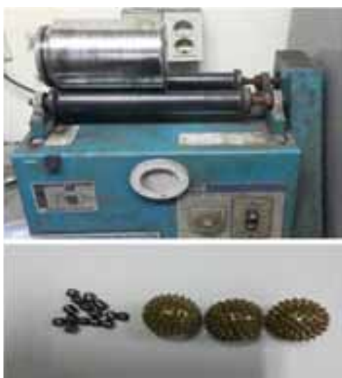
Fig. 2 Ball milling equipment and used milling balls
