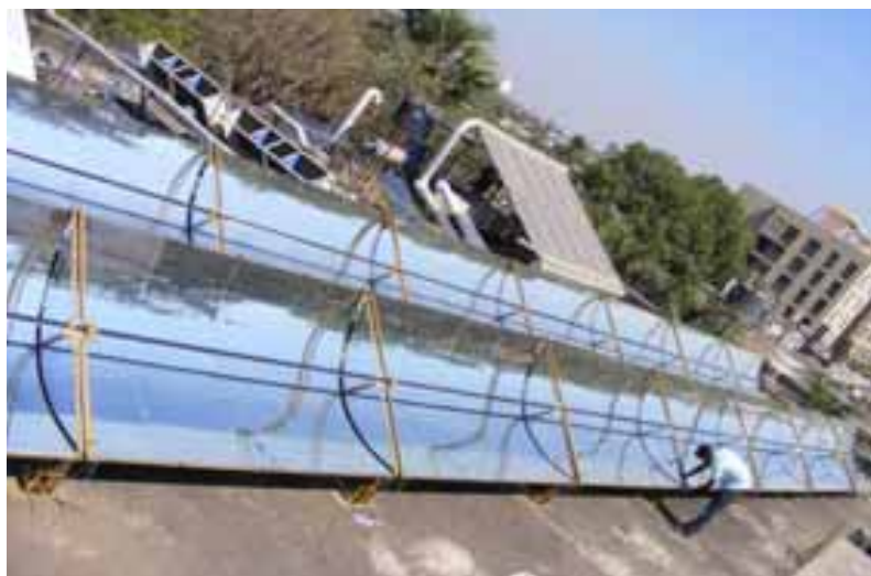
Fig. 3. A photo of the experimental 100 m 2 CPC system.
