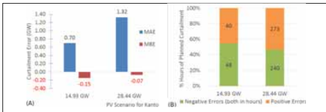
Fig. 3: Curtailment error with day-ahead regional forecasts for Kanto in two scenarios of PV power penetration (A), and frequency of curtailment errors according to their sign (B).
