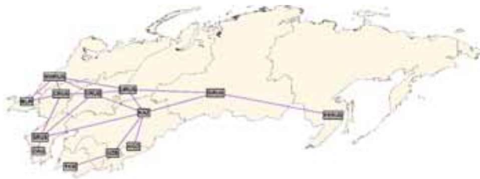
Fig.2. Eurasian sub-regions and HVDC transmission lines configuration.
