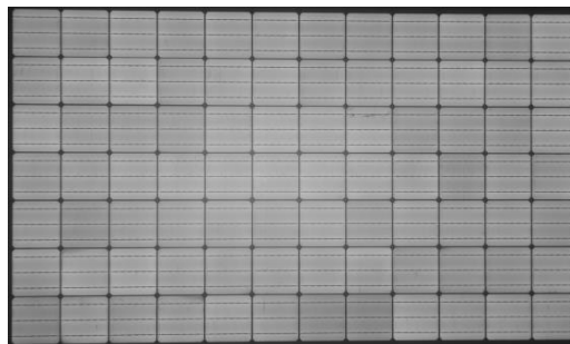
Figure 10: Electroluminescence picture of glass-glass photovoltaic modules without any cell cracks.
