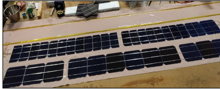
Fig. 3: Soldering of the bifacial-cell strings for the receivers.
