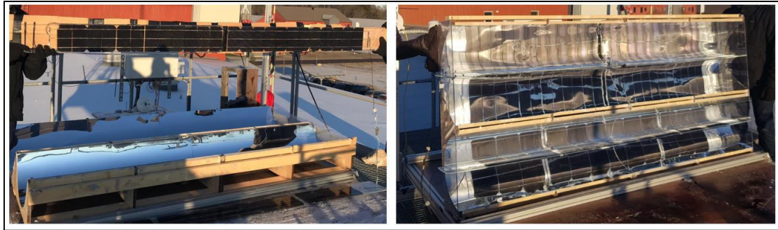
Fig. 5: Left side: testing receiver output outside the collector at 1X concentration. In this case, the receiver back face is covered as to test for the peak power contribution, mostly from DNI, of the front face. Right side: The receivers are placed inside the box and switched between the two concentration troughs to test for their output at 1.25X and 1.66X.
