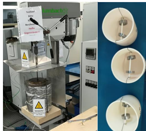
Fig. 3: Assembly of Flow Acceleration Corrosion test and corrosion by gravimetry
