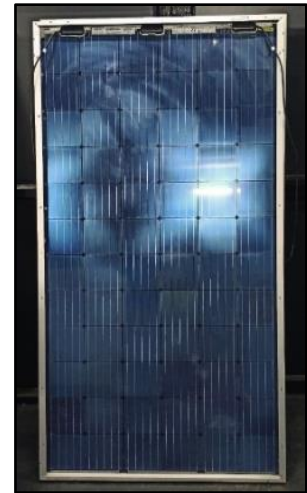
Fig. 9: Standard frame shading the rear side of a bPV module
