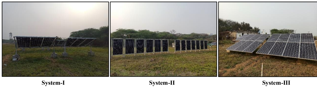
Fig. 1: System-I: bPV system at Latitude Tilt, System-II: bPV system at Vertical Tilt, System-III: mPV system at Latitude Tilt
