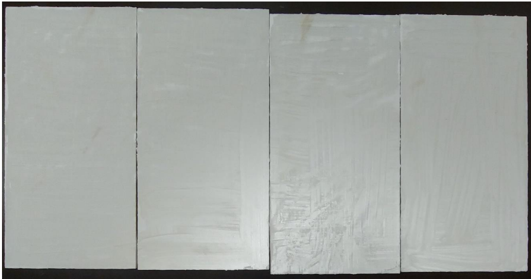
Fig. 1: The four retroreflective panels used in the measurements.
