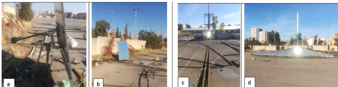
Figure 8: Different views of the solar concentration system showing the solar reflection. (a) Reflector and the tracking mechanism from the side (b) Reflector front view supported from behind (c) Reflection of solar thermal radiation on the tower base (d) Front view of the system with collector extending towards south
