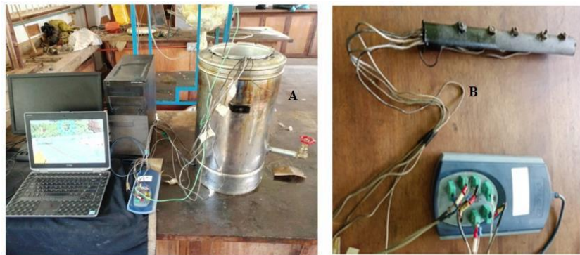
Figure 2: A) Showing the picture of the experimental setup of single tank system integrated with a cooking unit B) is the positioning of thermocouples and Pico data logger.
