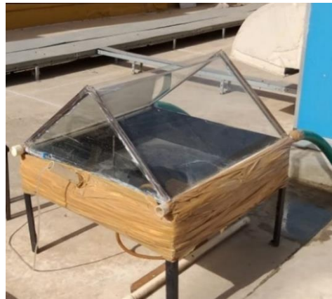
Figure 2: A photograph of double-slope, passive solar still (MUJ, Jaipur, India)
